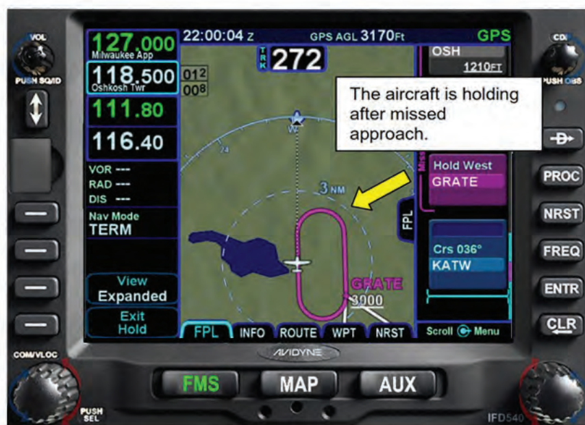
Figure 9 - 26 Holding After the VOR 27 Approach
