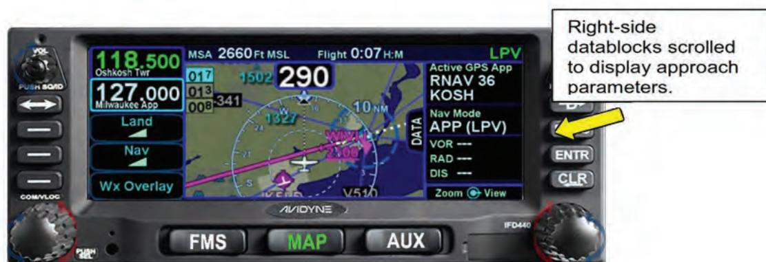
Figure 11 - 43 IFD440 Right Side Datablocks
