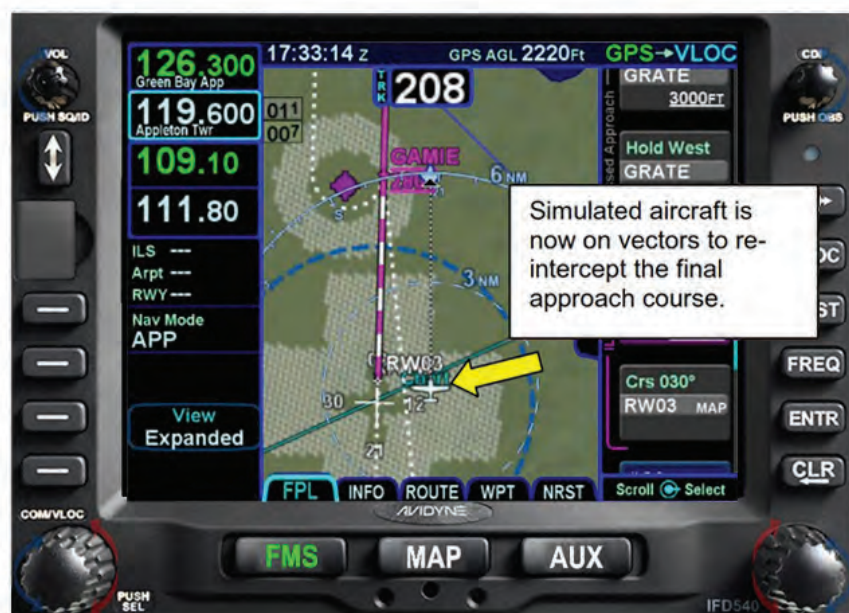
Figure 9 - 32 ILS Approach After Reactivation
