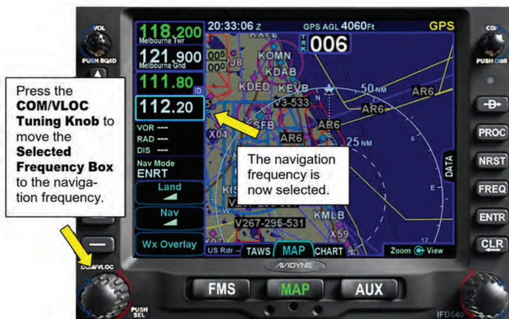
Figure 3 - 8 Selecting a Nav Frequency Box
