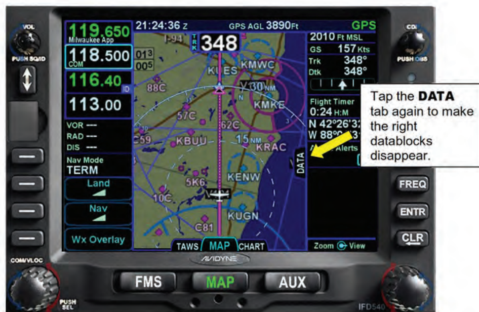
Figure 4 - 28 Removing the Right Datablocks
