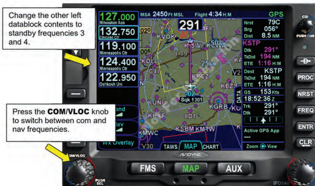
Figure 11 - 14 IFD540 Set Up with Four Standby Frequencies
