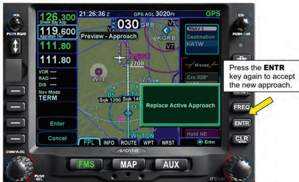
Figure 9 - 16 Confirming the New Approach
