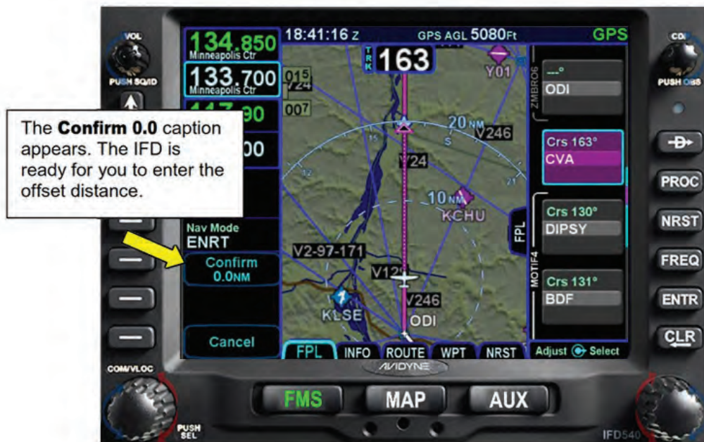
Figure 6 - 37 The Offset Route Distance Box
