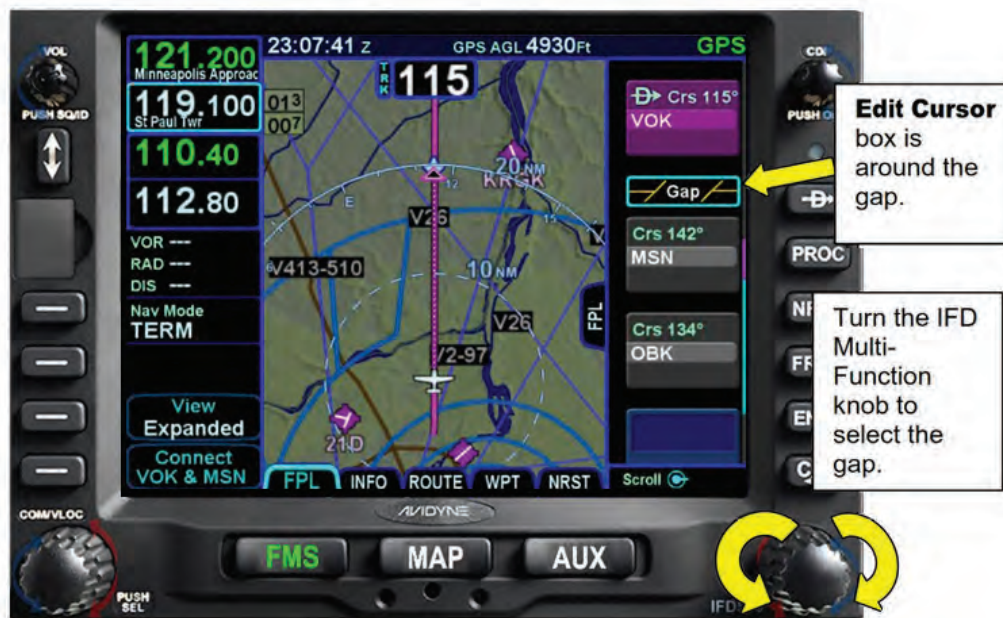
Figure 5 - 13 Selecting the Flight Plan Gap
