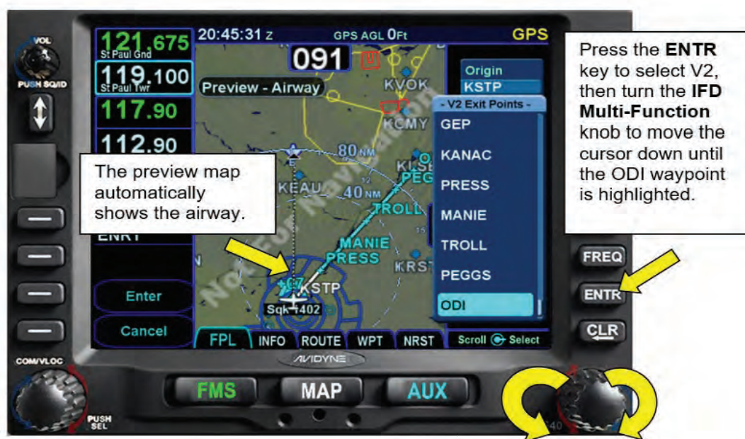
Figure 6 - 3 Selecting the Airway Exit Point
