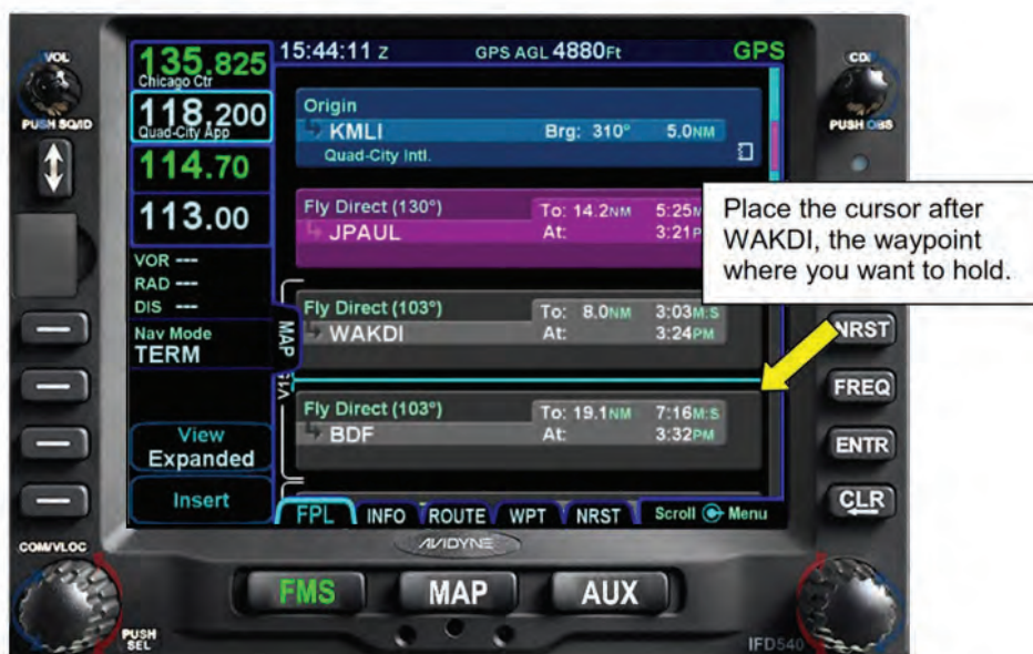
Figure 8 - 2 The Insertion Point for the Holding Pattern
