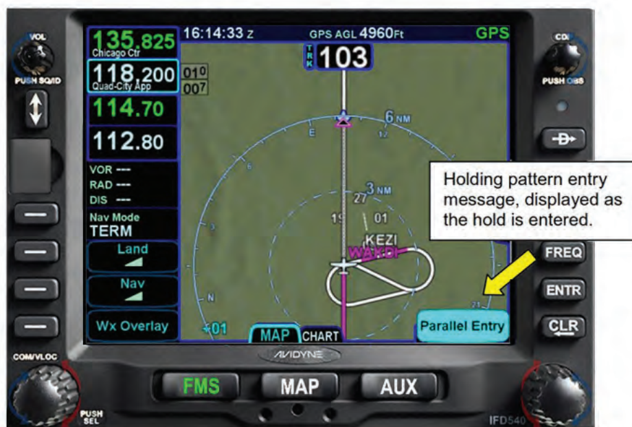
Figure 8 - 10 Holding Pattern Entry Message
