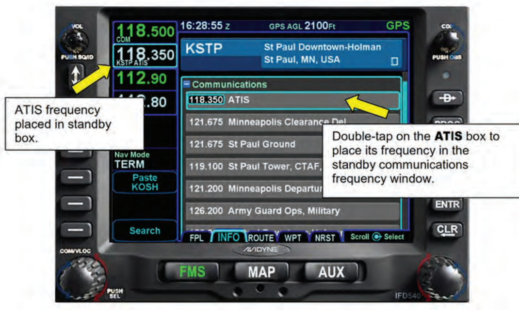
Figure 10 - 10 Loading the ATIS Frequency
