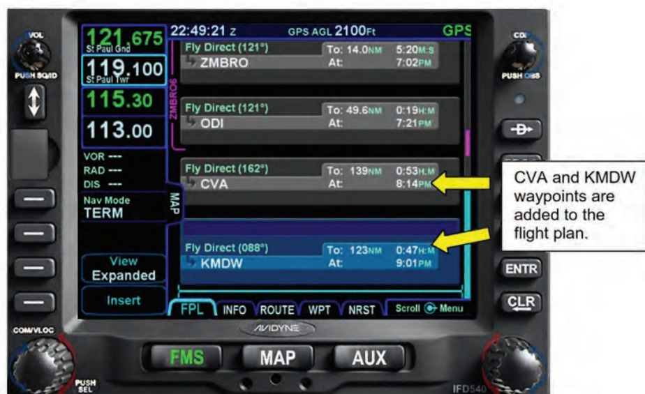
Figure 6 - 20 Flight Plan Before Arrival Is Added
