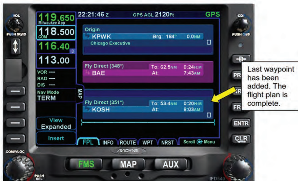
Figure 4 - 13 Completed Flight Plan
