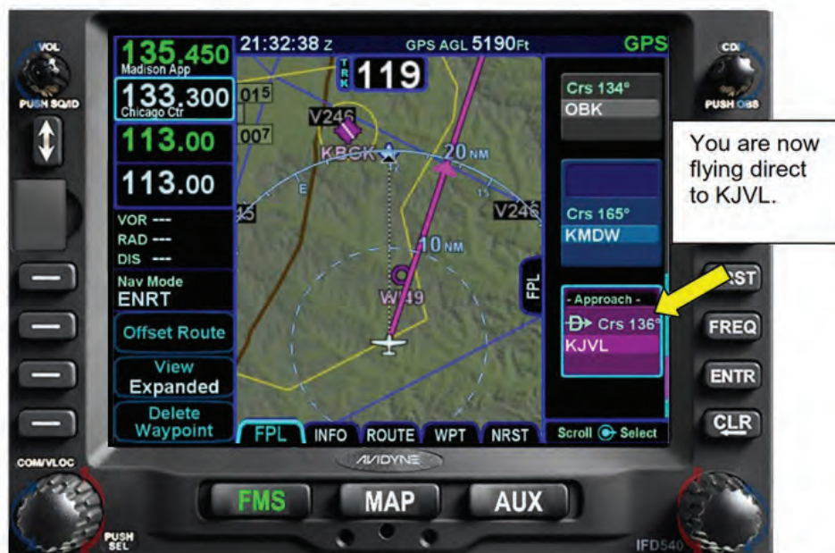
Figure 5 - 26 Flight Plan to New Destination
