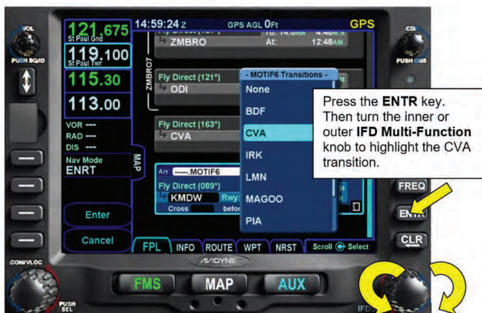
Figure 6 - 23 Selecting the Transition Route
