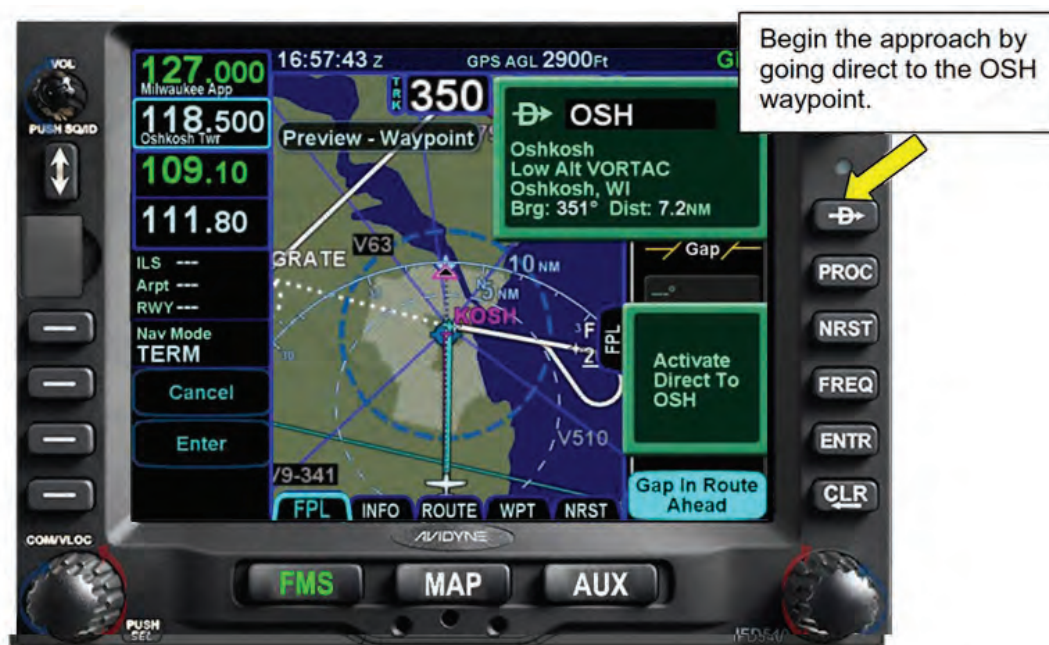
Figure 9 - 23 Going Direct to the Initial Approach Fix
