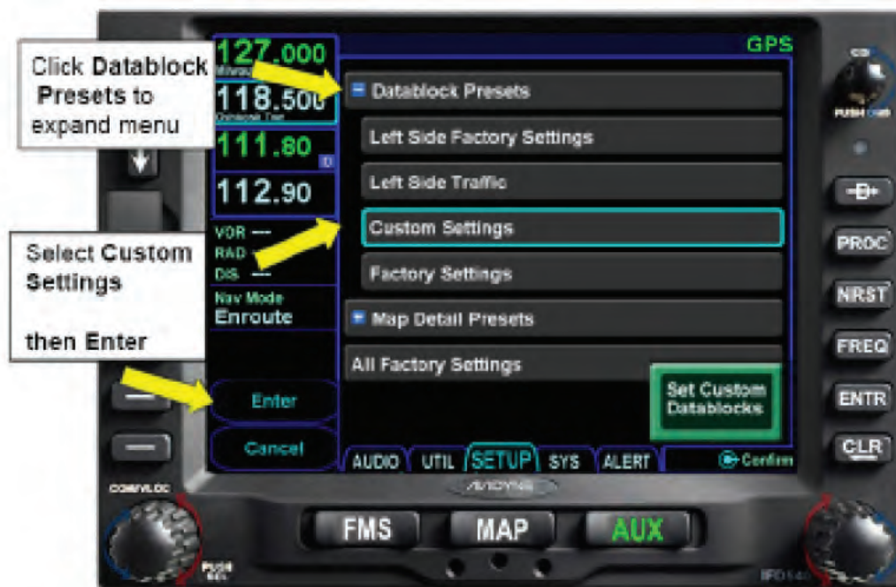
Figure 11 - 5 Selecting a Datablock to Edit
