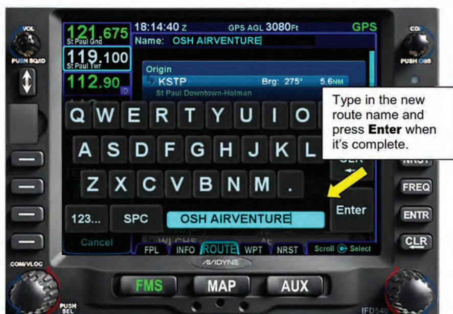
Figure 7 - 5 Keying in the New Route Name
