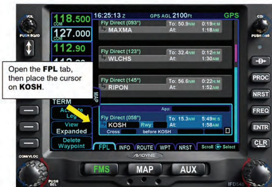
Figure 10 - 6 Selecting the Destination Airport
