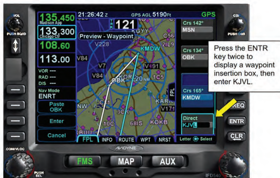
Figure 5 - 24 Entering the New Destination Waypoint
