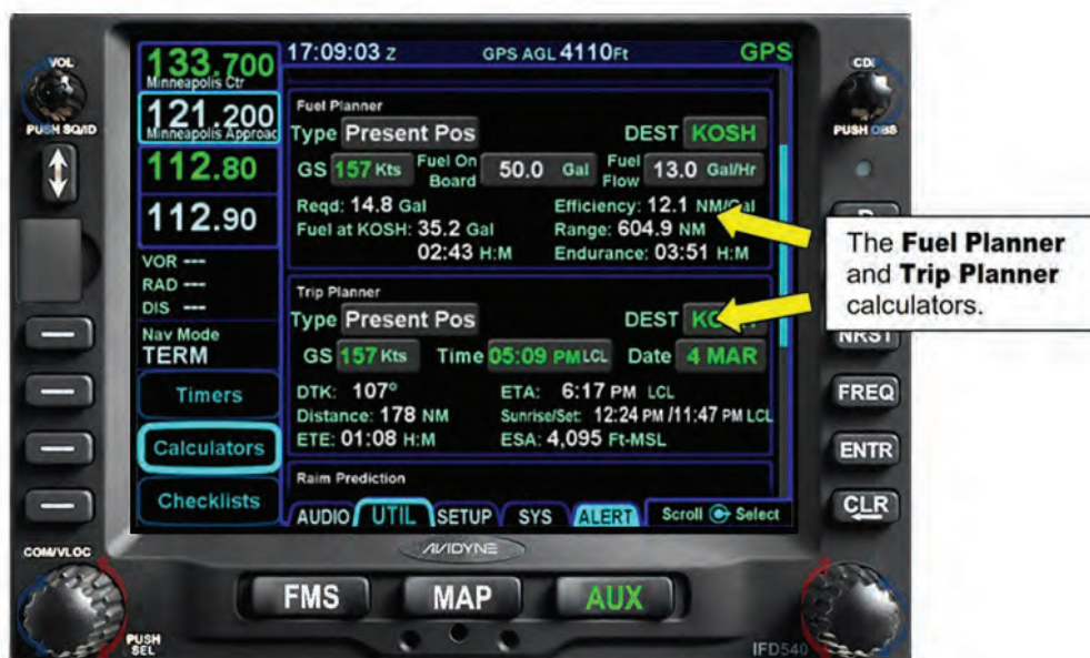
Figure 10 - 31 The Fuel and Trip Planner Calculators
