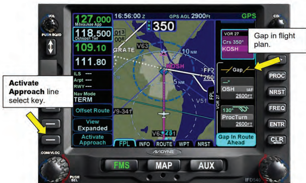
Figure 9 - 22 The Gap in the Flight Plan
