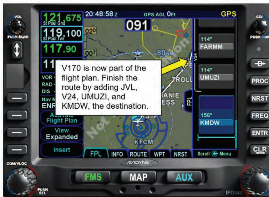
Figure 6 - 7 Completed Flight Plan with Airways
