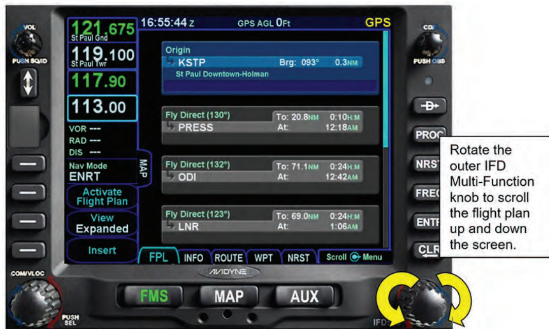
Figure 5 - 1 The Completed KSTP-KMDW Flight Plan
