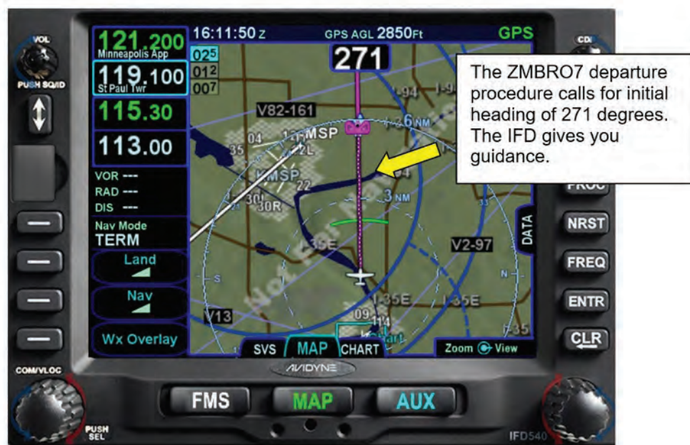
Figure 6 - 27 Initial Leg of Departure
