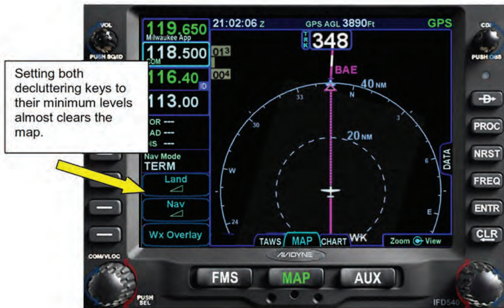
Figure 4 - 24 Maximum De-Cluttering
