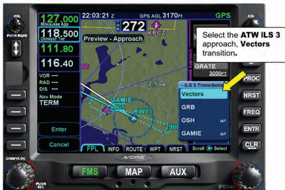
Figure 9 - 27 Selecting the ILS 3 Approach to KATW
