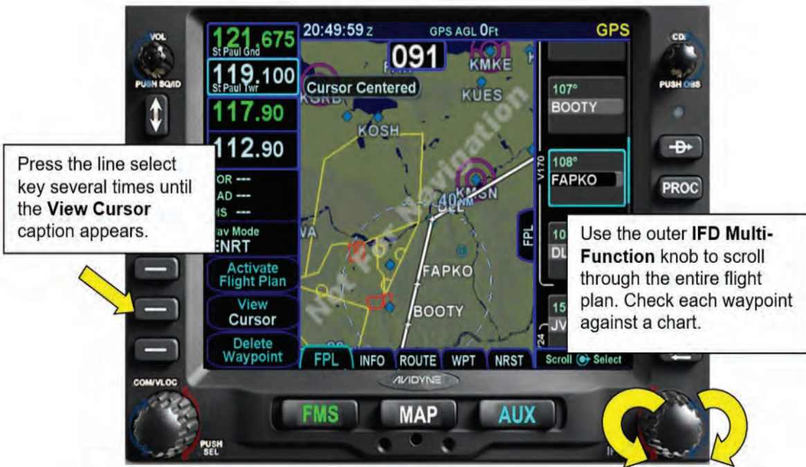
Figure 6 - 8 Reviewing the Flight Plan with View Cursor
