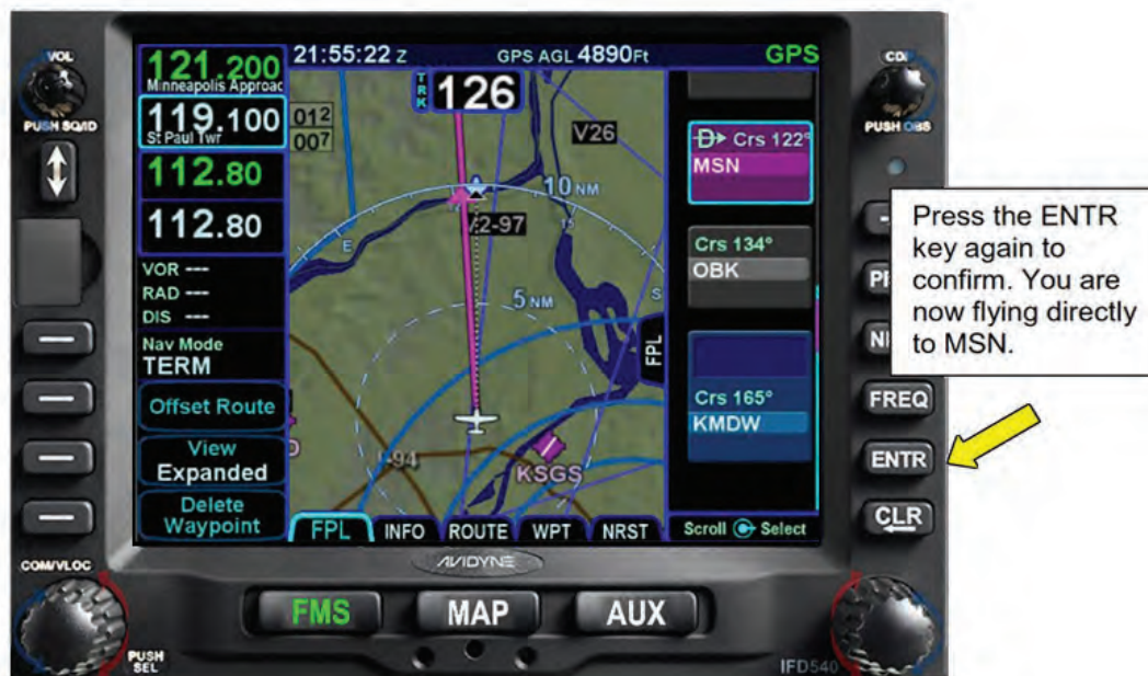
Figure 5 - 10 Entering a New Direct-To Waypoint
