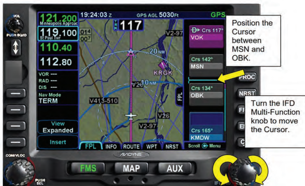
Figure 5 - 17 Positioning the Insert Cursor
