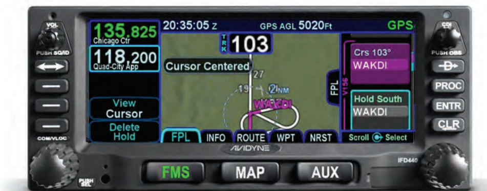
Figure 8 - 25 IFD440 Holding Pattern Display
