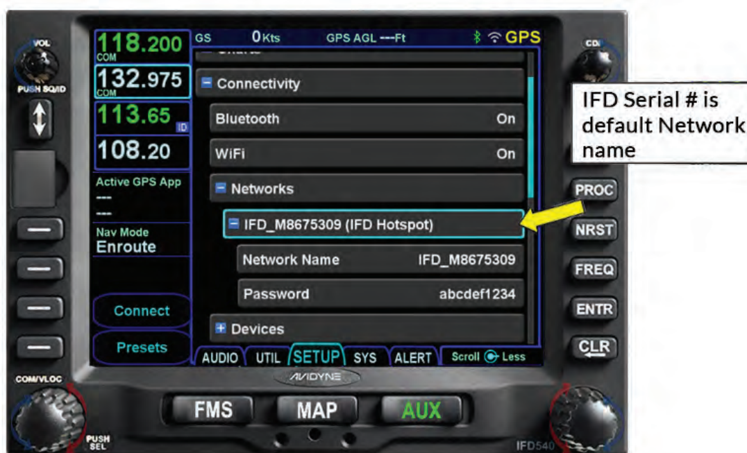
Figure 11 - 36 IFD Network- Default Name & Password
