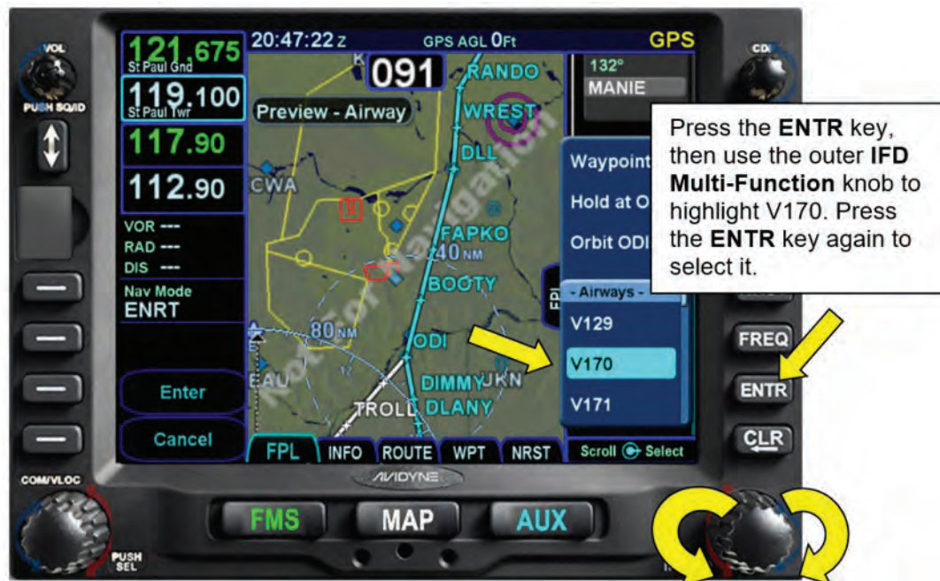
Figure 6 - 5 Selecting the Next Airway
