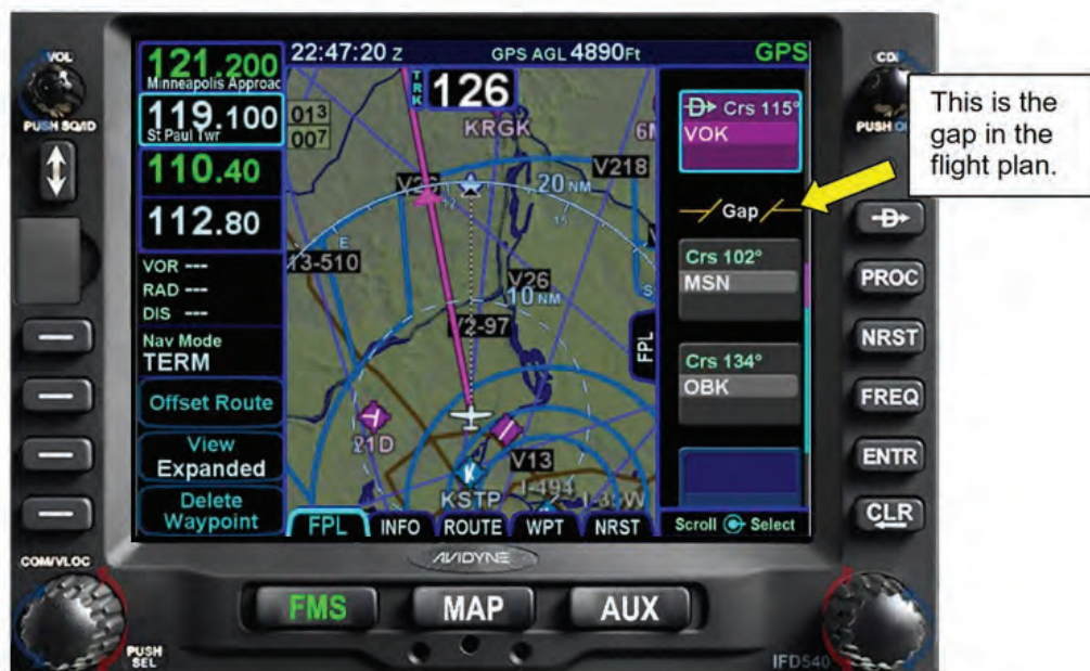
Figure 5 - 12 Flight Plan Gap
