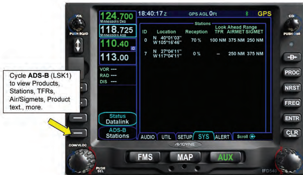
Figure 10 - 45 Displaying Datalink Information
