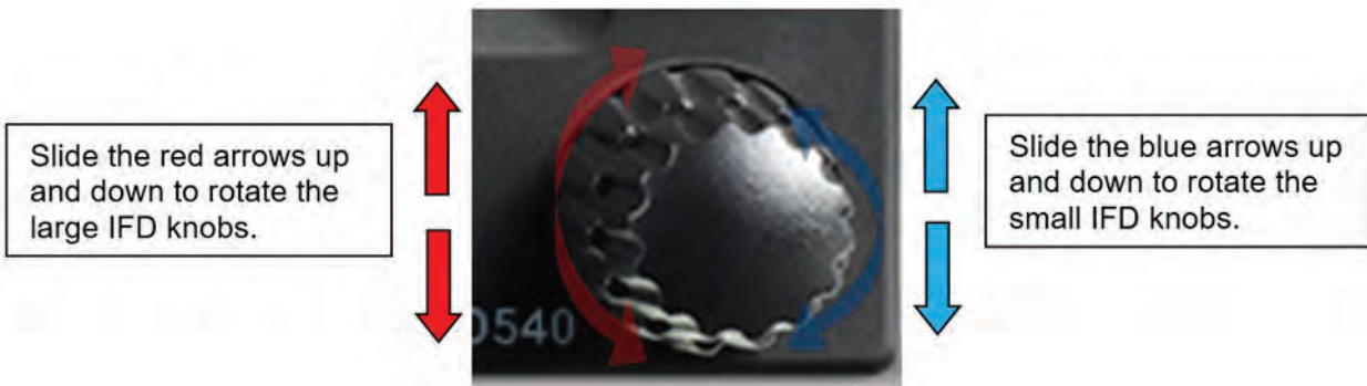
Figure 2 - 7 IFD Knob Operation
