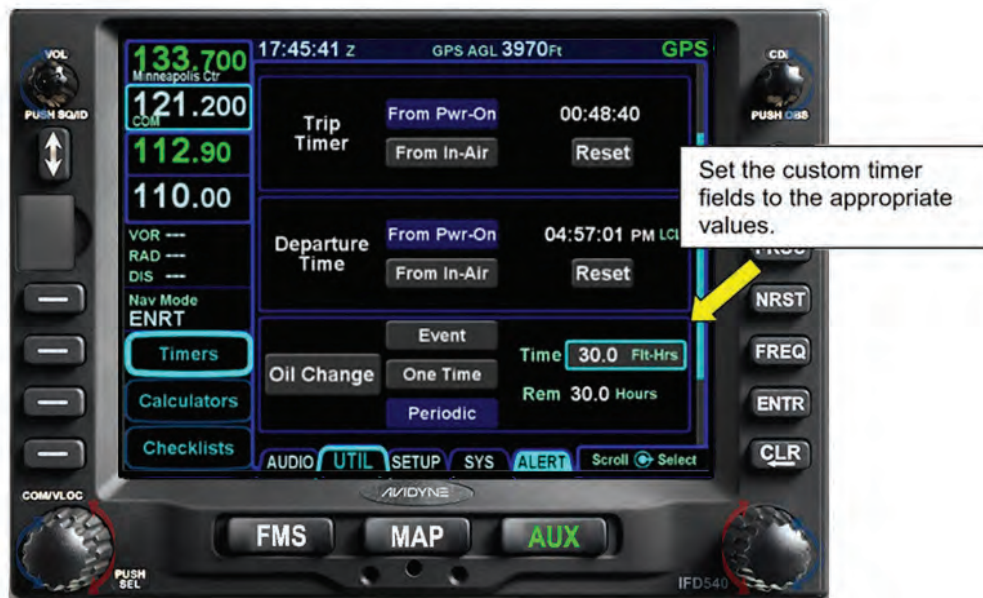
Figure 10 - 27 Setting Field Values for a Custom Timer
