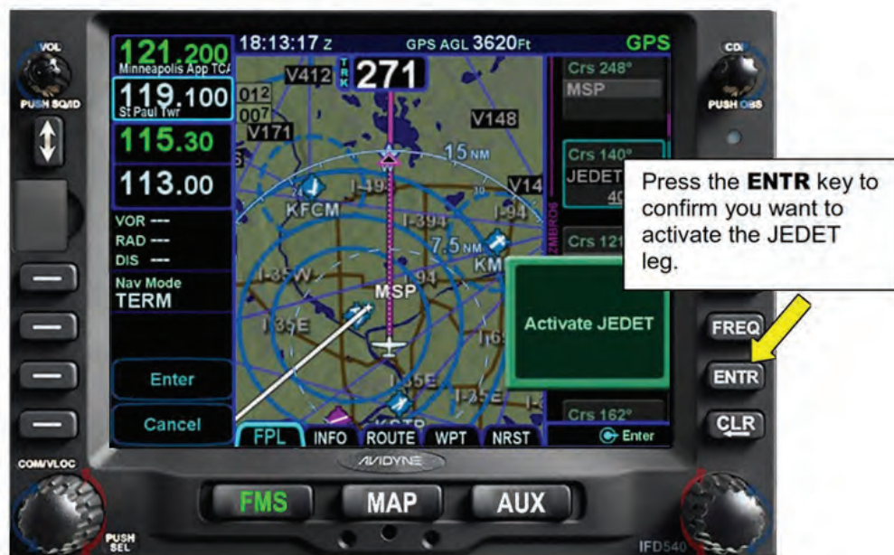
Figure 6 - 29 Activating the Second Departure Leg
