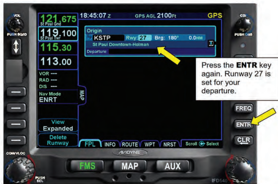
Figure 6 - 14 Completed Departure Runway
