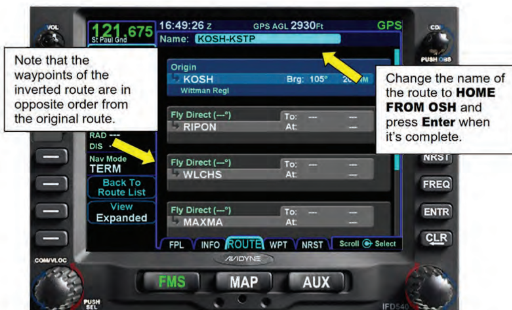
Figure 7 - 9 The Inverted Route
