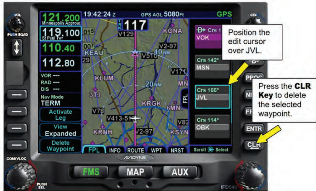
Figure 5 - 21 Deleting a Waypoint
