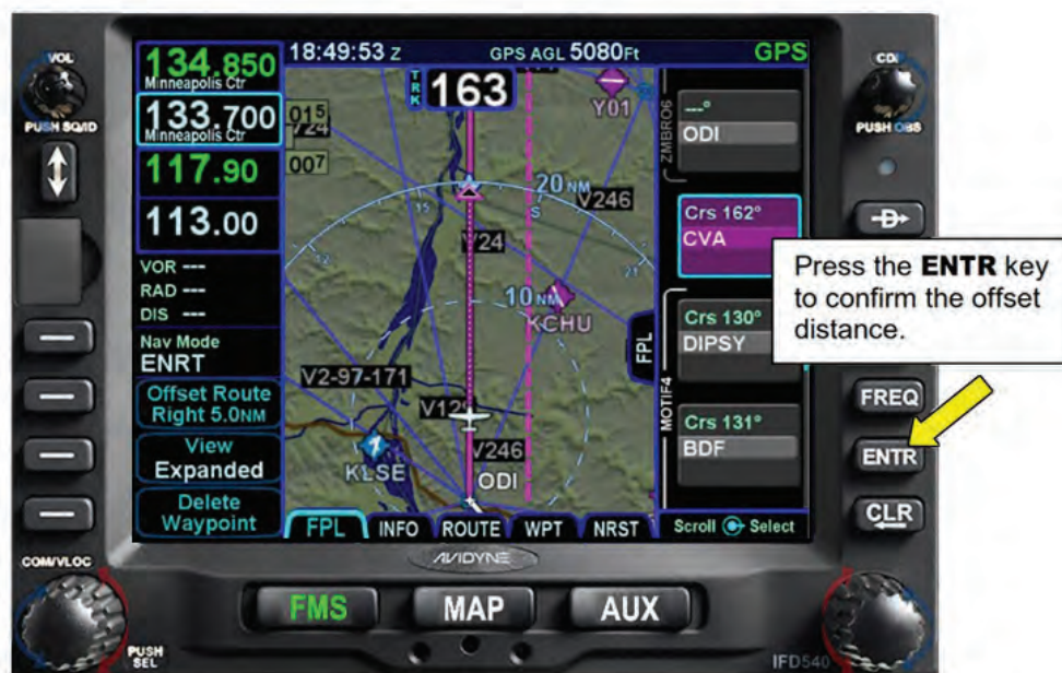
Figure 6 - 39 Confirming the Offset
