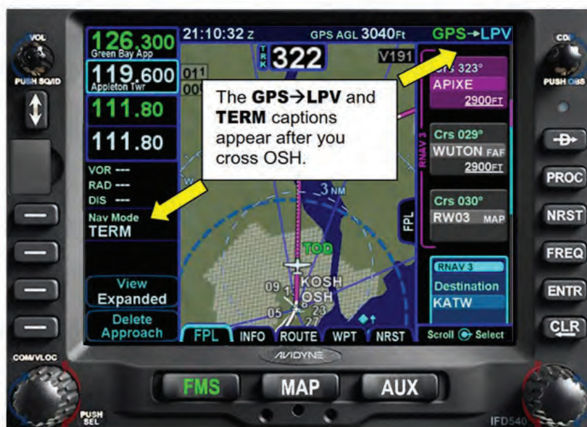
Figure 9 - 11 Indications on First Part of Approach
