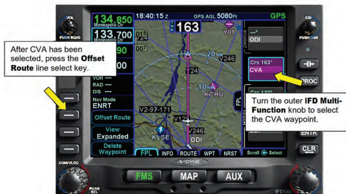
Figure 6 - 36 Selecting the Leg to Offset
