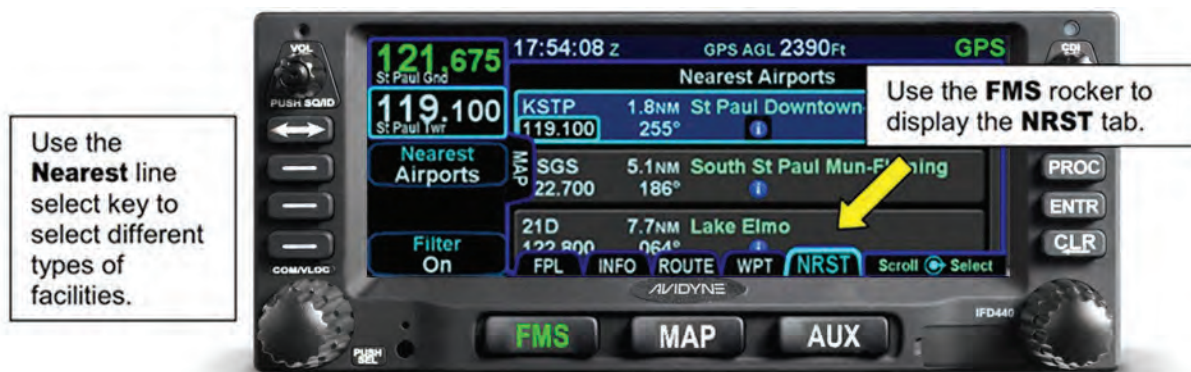
Figure 10 - 46 Displaying the NRST Tab on the IFD440
