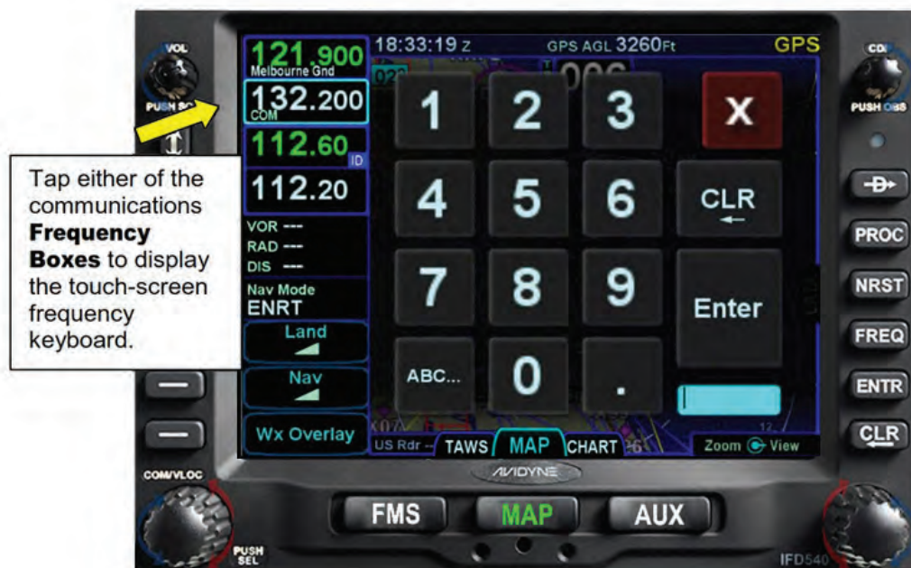
Figure 3 - 5 Bringing Up the On-Screen Keyboard
