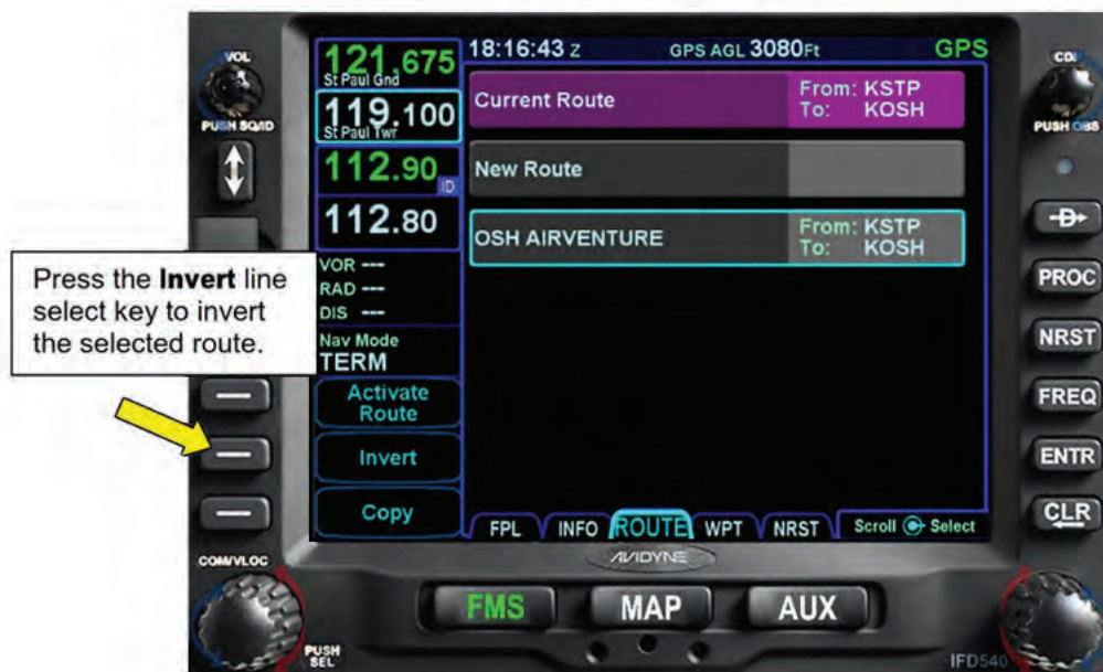
Figure 7 - 8 Using the Invert Line Select Key
