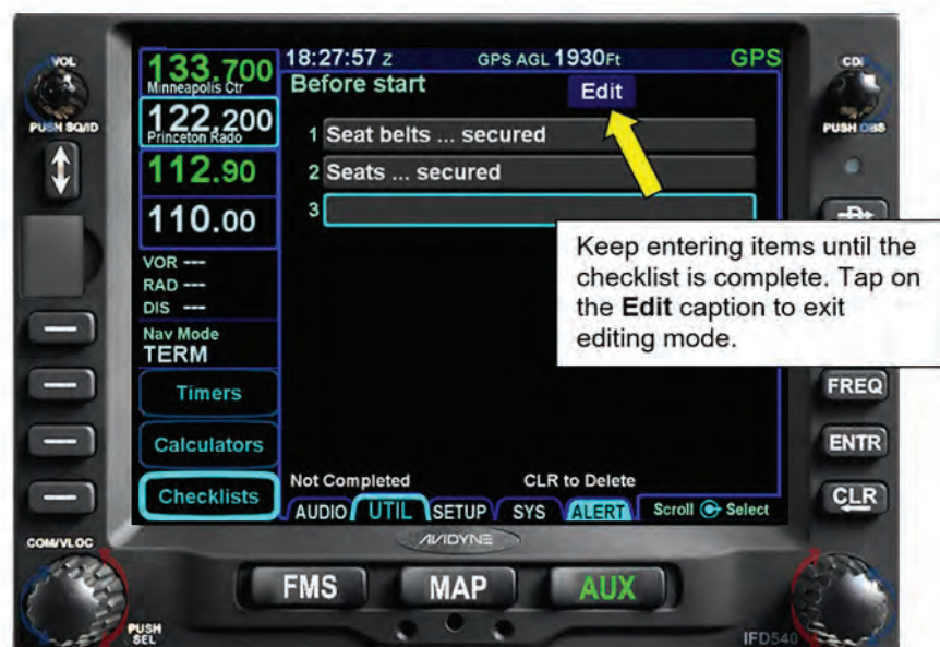
Figure 10 - 37 Checklist After Two Items Have Been Entered
