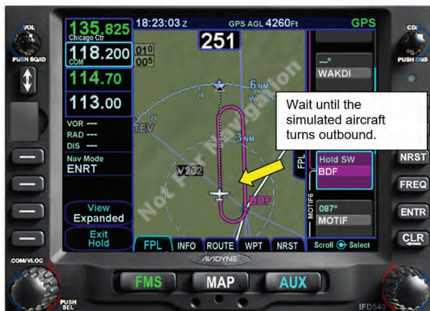
Figure 8 - 21 Aircraft in Position For Exit of BDF Hold
