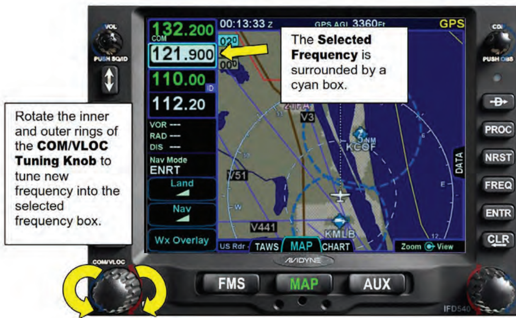
Figure 3 - 3 Changing a Communications Frequency
