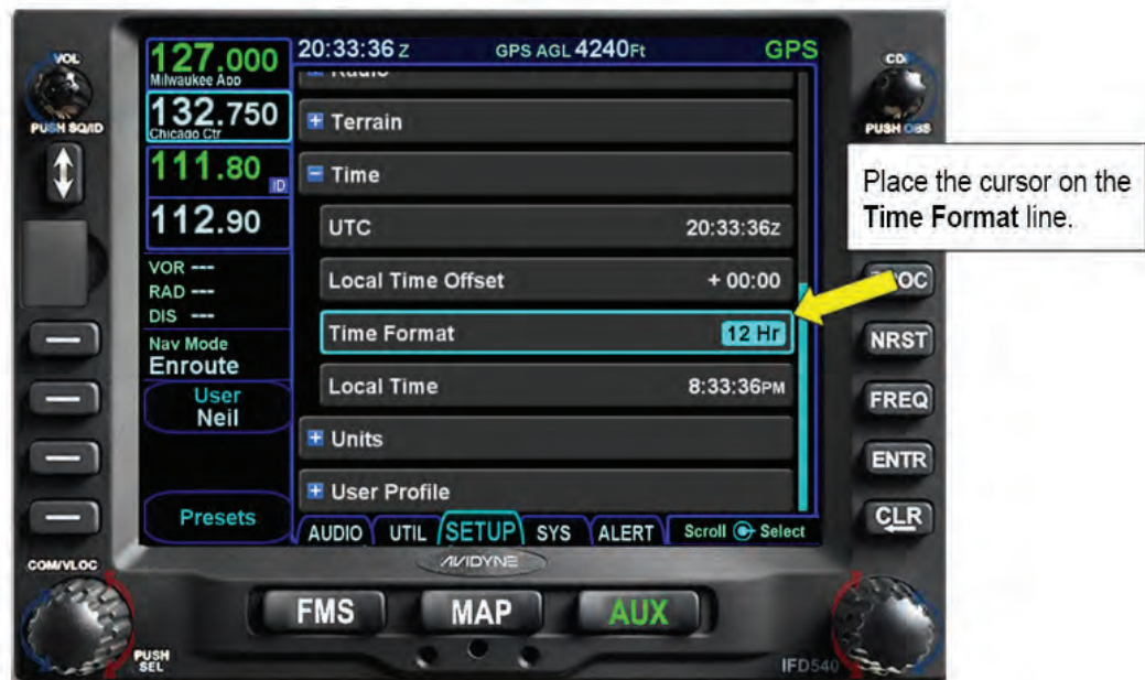
Figure 11 - 30 Selecting the Time Format Line
