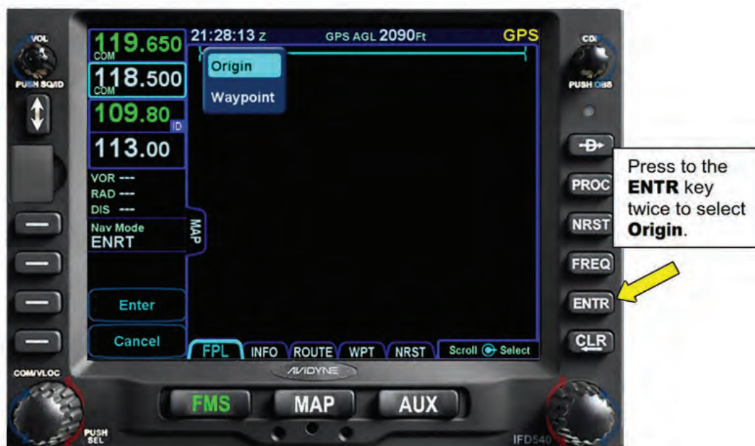
Figure 4 - 4 Flight Plan Origin
