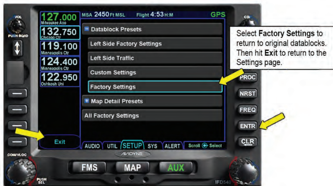
Figure 11 - 15 Returning to the Factory Default Datablocks
