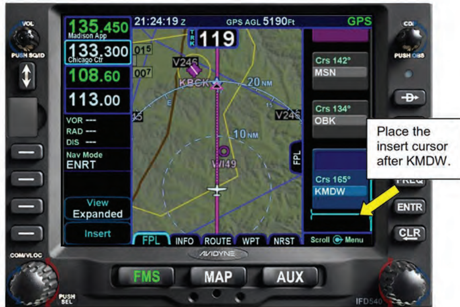
Figure 5 - 23 Positioning the Insert Cursor at the End of the Flight Plan
