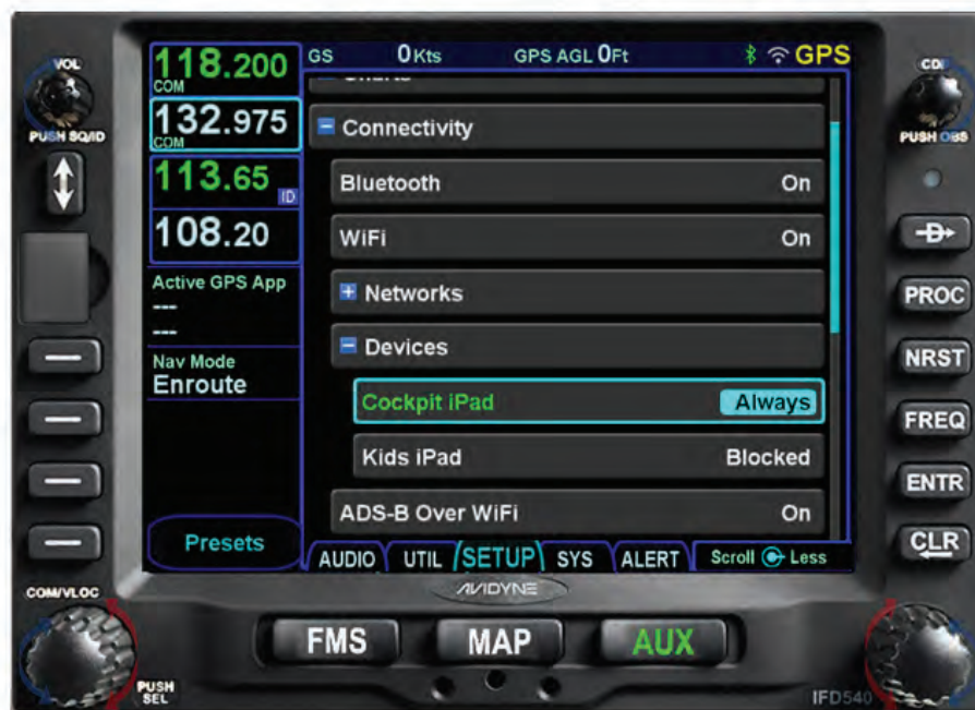
Figure 11 - 38 Devices - Enable the device(s) you want connected to your IFD.
