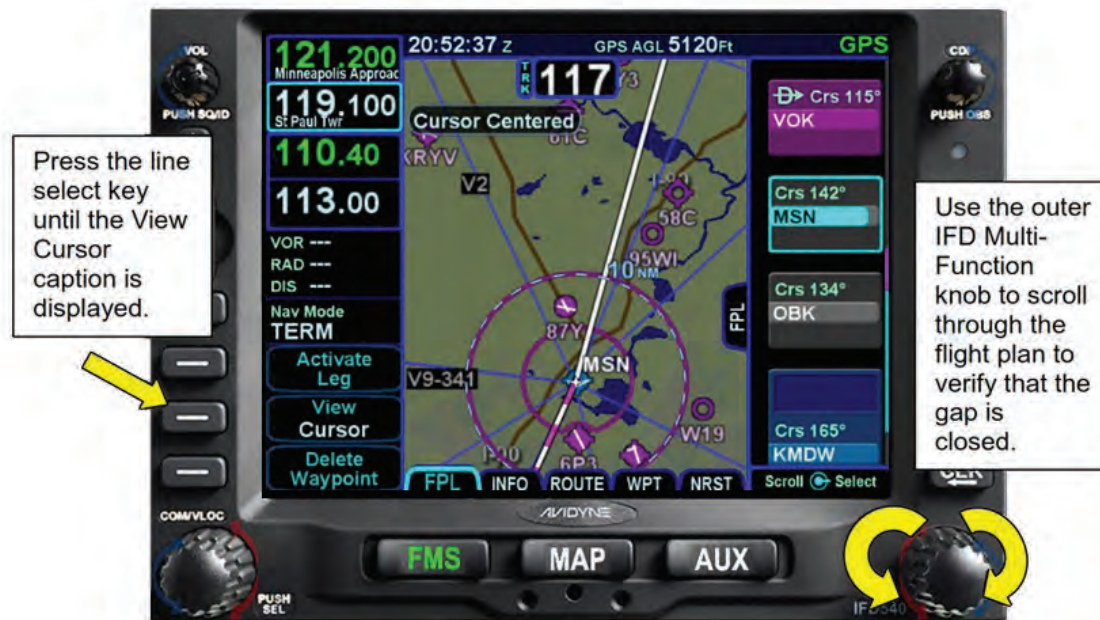
Figure 5 - 16 Reviewing the Flight Plan
