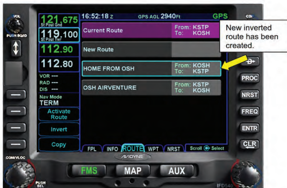
Figure 7 - 10 Route List with Both New Routes
