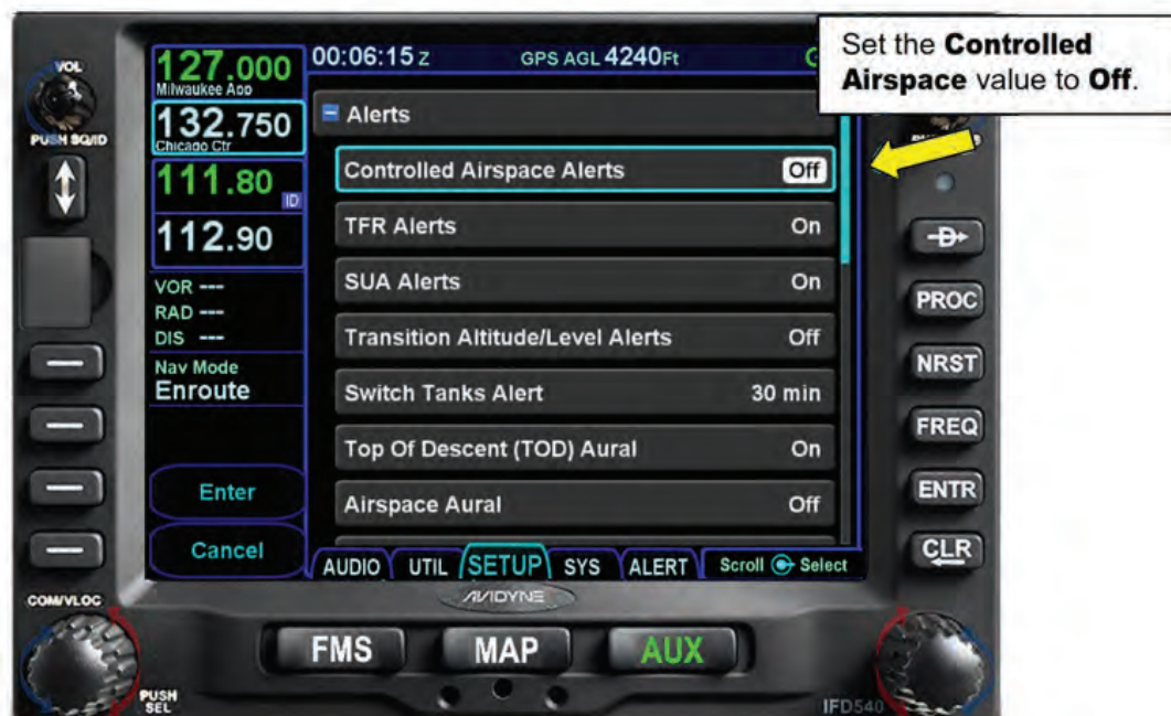
Figure 11 - 16 Controlling Airspace Alerts
