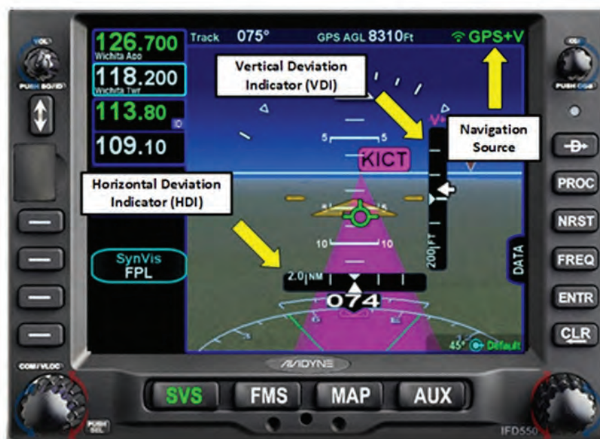
Figure 6 - 46 VNAV Guidance on SVS Page (IFD550/545)
