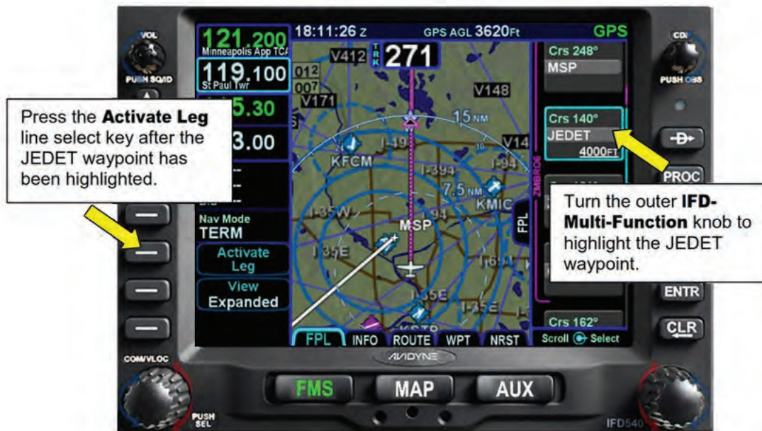
Figure 6 - 28 Selecting the Second Departure Leg
