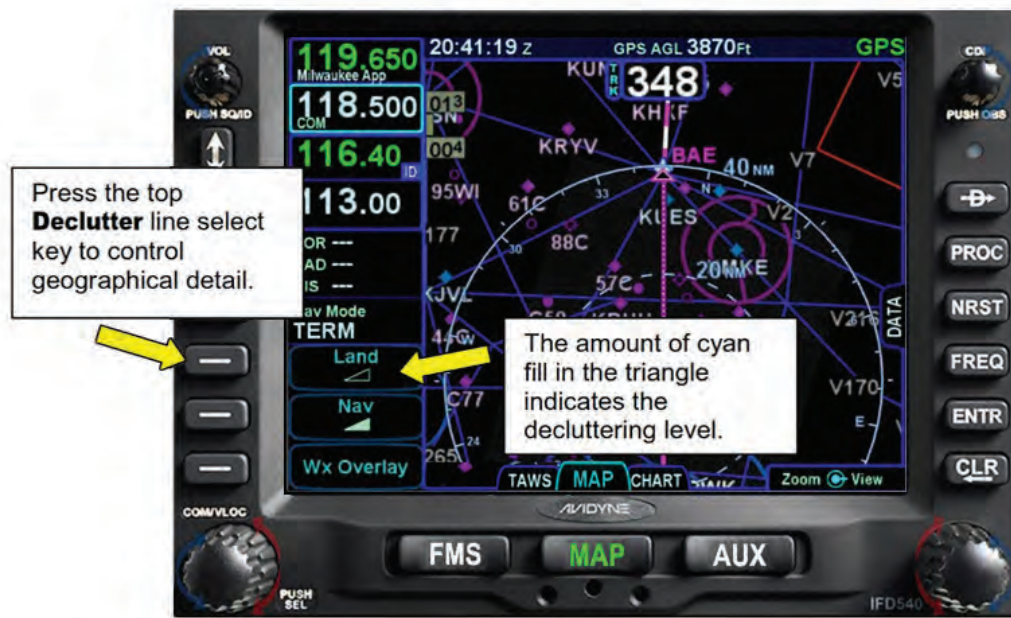
Figure 4 - 22 The Land De-Cluttering Key
