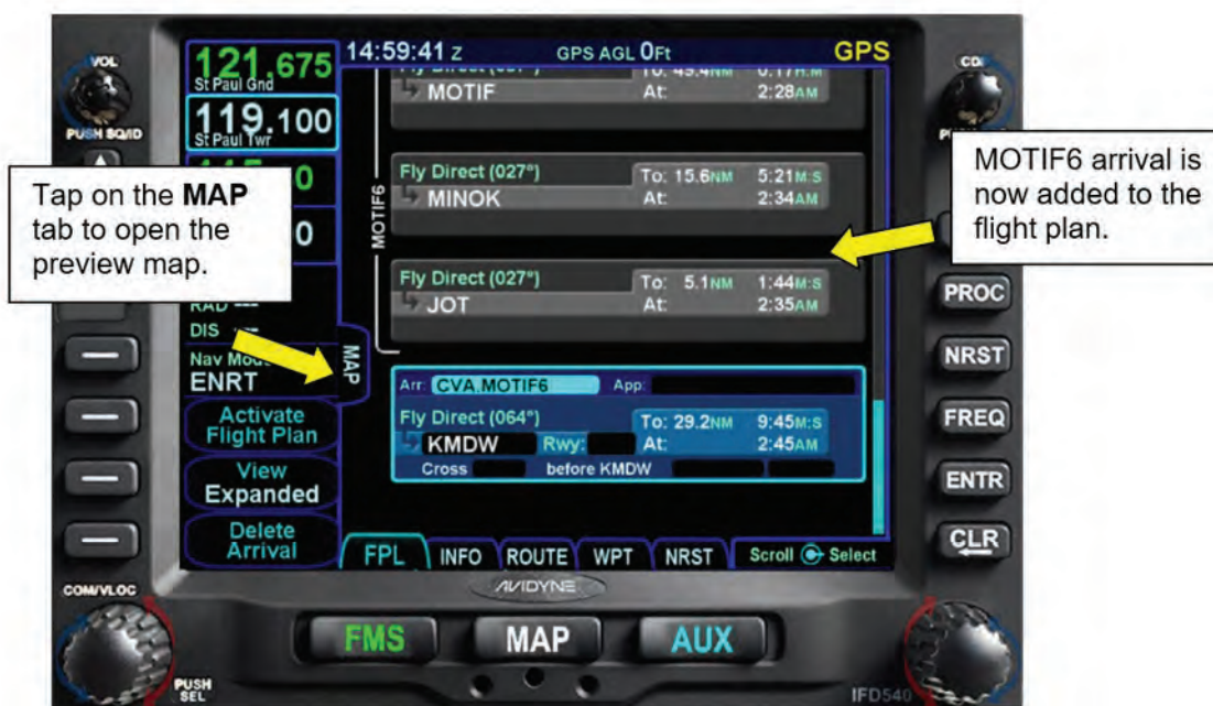
Figure 6 - 24 MOTIF6 CVA Transition Added to Flight Plan
