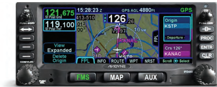
Figure 5 - 27 IFD440 Flight Plan MAP Tab Display
