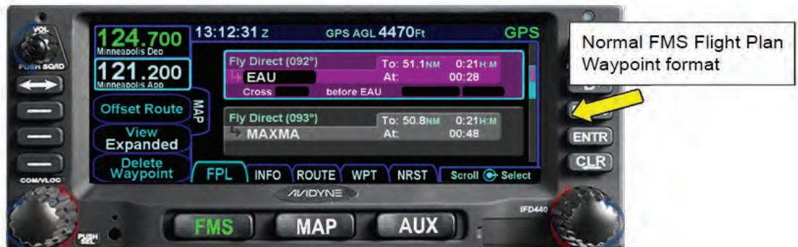
Figure 11 - 44 IFD440 Normal FMS Waypoint format on FMS FPL page
