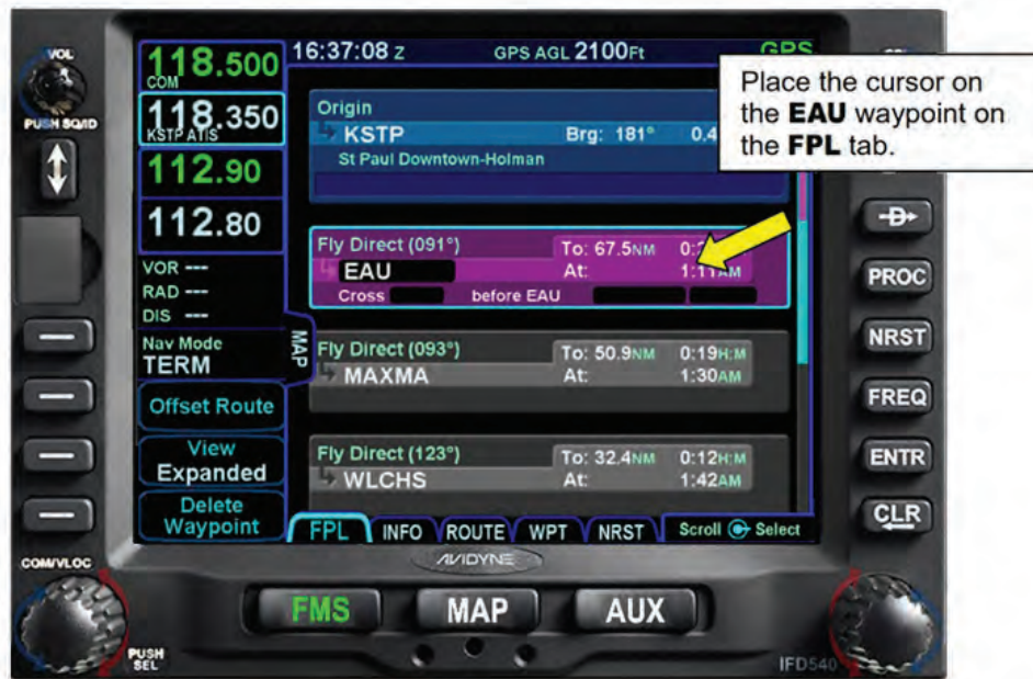
Figure 10 - 12 Selecting the EAU Waypoint
