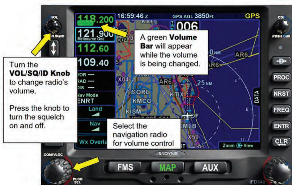
Figure 3 - 13 Controlling Volume and Squelch
