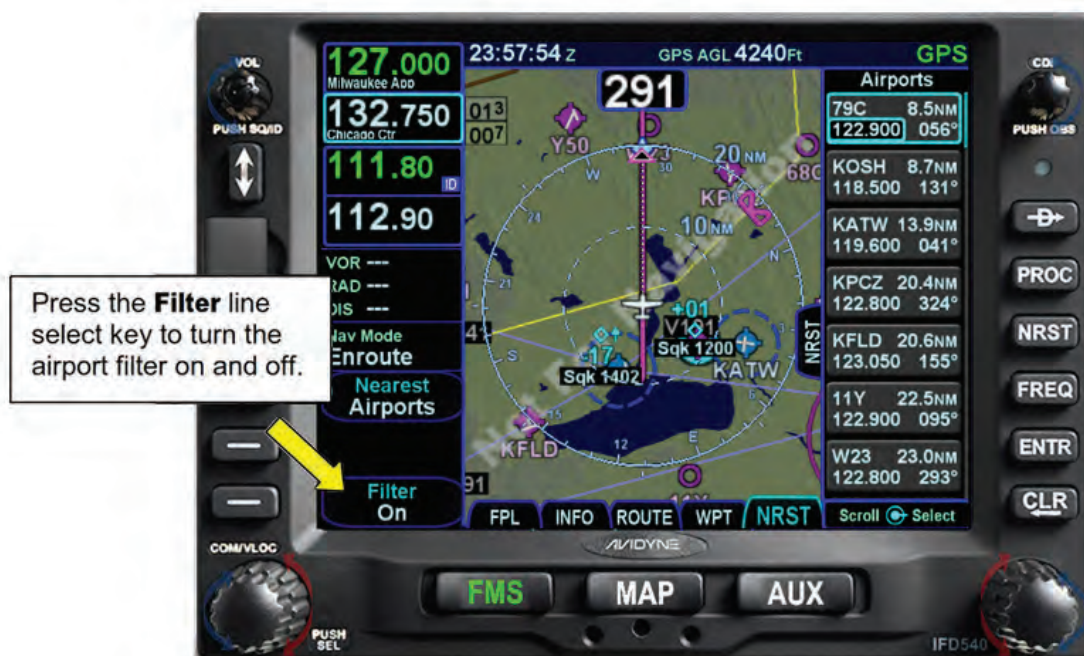
Figure 11 - 23 Turning the Runway Filter On and Off
