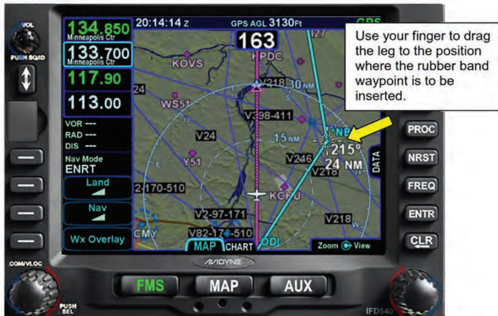
Figure 6 - 43 Using Rubber Band Mode to Offset a Flight Plan Leg
