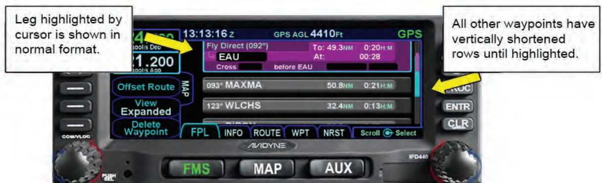
Figure 11 - 46 Mini Flight Plan Format on FMS FPL page
