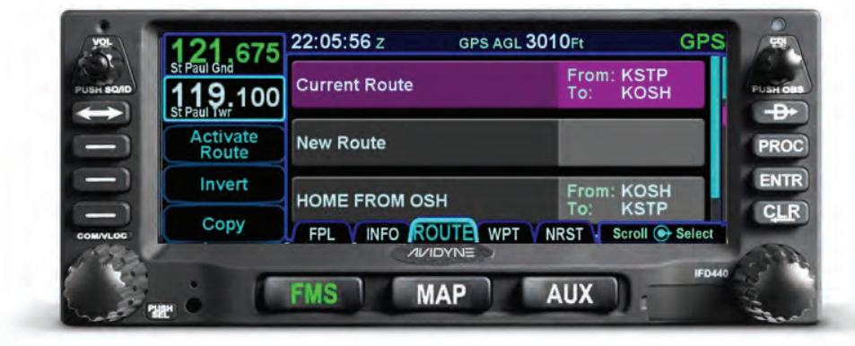
Figure 7 - 22 IFD440 Route Tab
