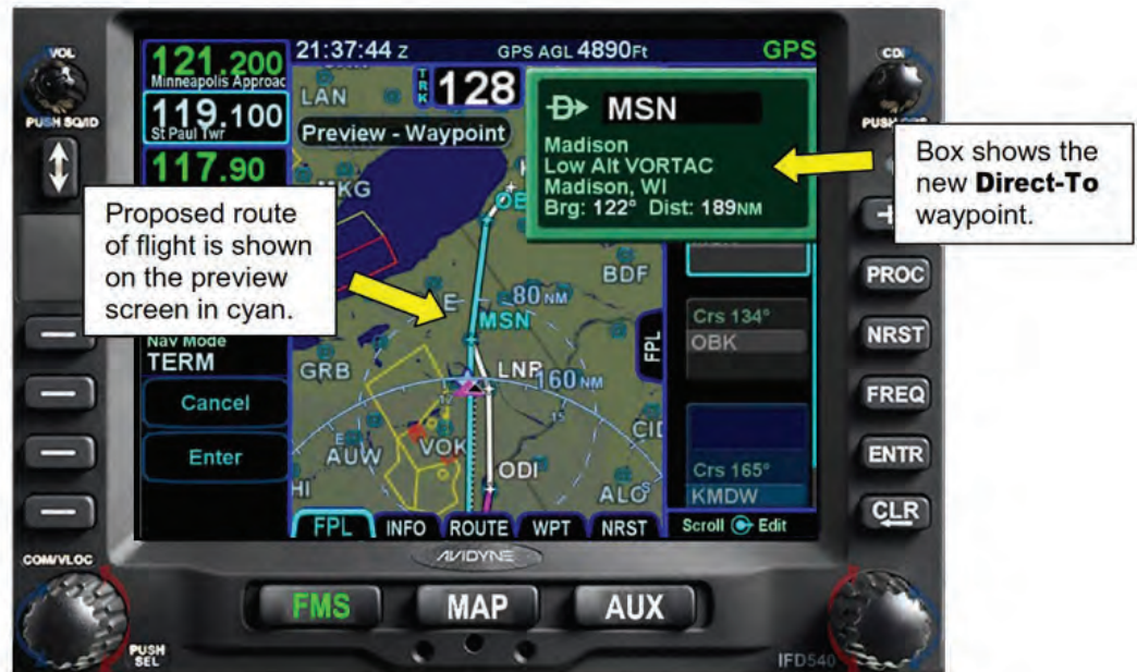
Figure 5 - 7 Previewing the Direct-To Waypoint
