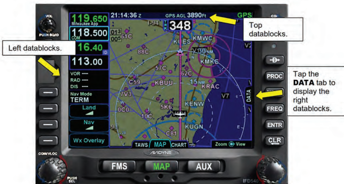
Figure 4 - 25 Displaying the Datablocks
