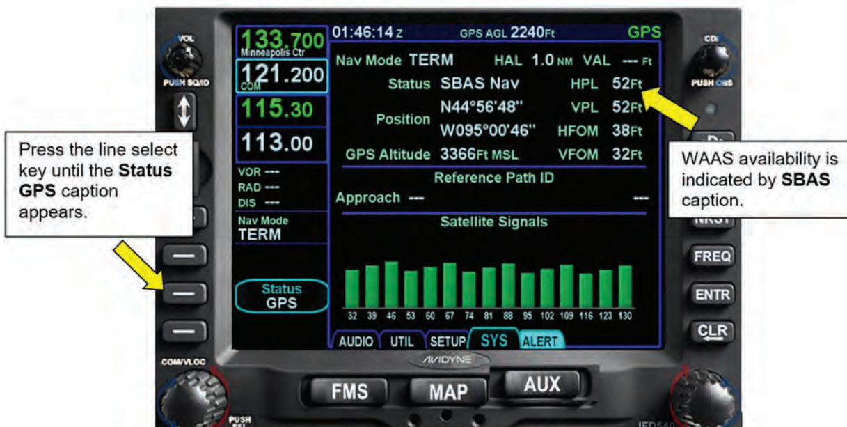
Figure 10 - 43 Displaying Nav Status Information
