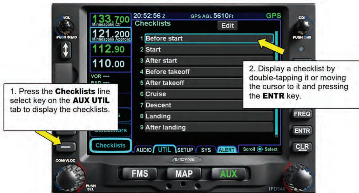
Figure 10 - 38 Displaying the Electronic Checklists
