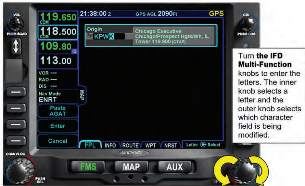
Figure 4 - 5 Entering the Origin Waypoint ID
