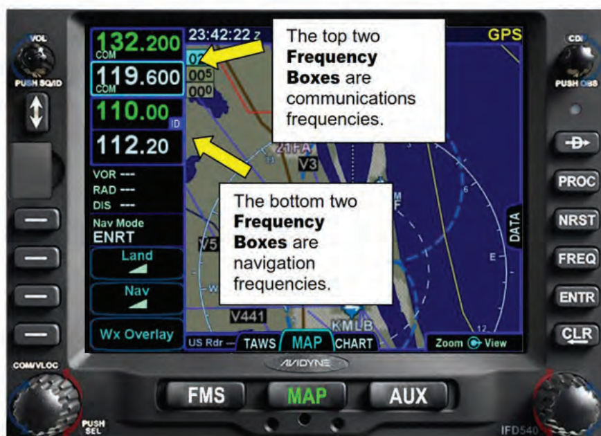
Figure 3 - 1 The IFD Com and Nav Frequency Boxes
