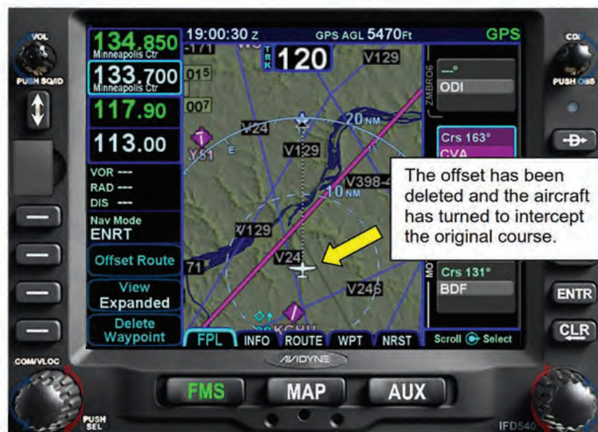
Figure 6 - 42 Flight Plan after Cancellation of Course Offset
