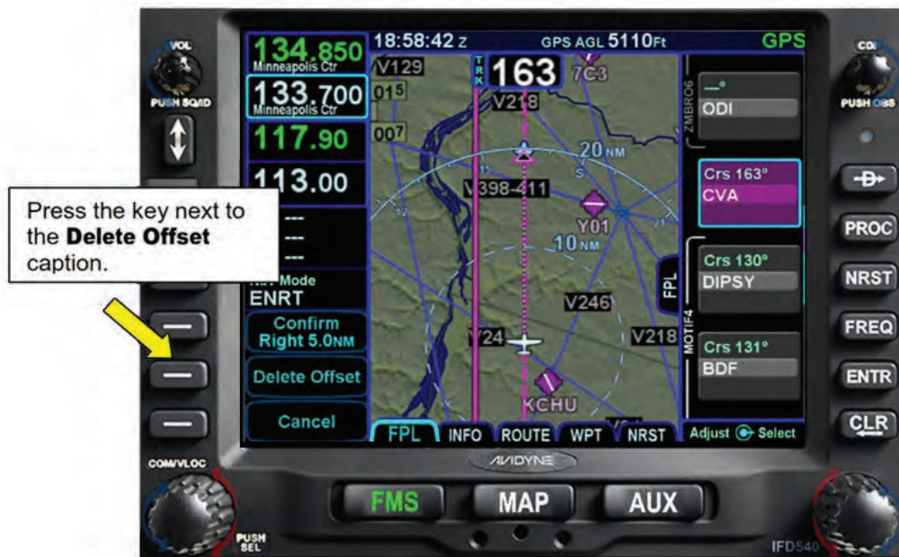
Figure 6 - 41 Confirming the Offset Cancellation
