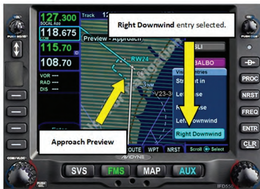
Figure 9 - 39 Right Downwind Entry Selected
