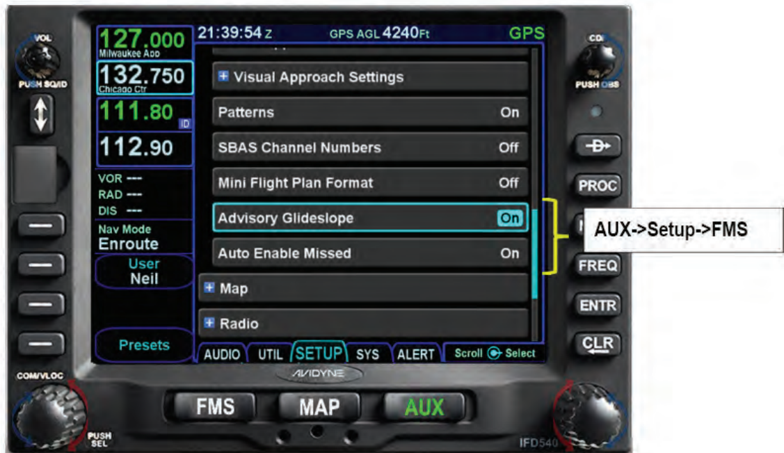
Figure 11 - 18 The Approach Settings - FMS related
