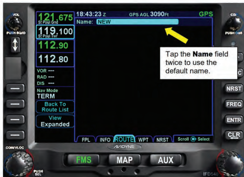
Figure 7 - 14 Using the Default Route Name
