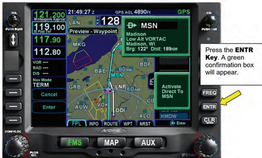
Figure 5 - 8 Activating the Direct-To Waypoint
