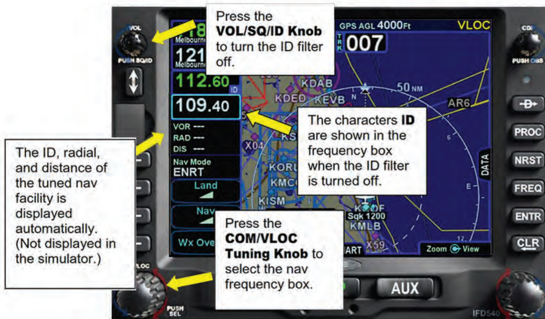
Figure 3 - 14 Checking the Nav Facility ID
