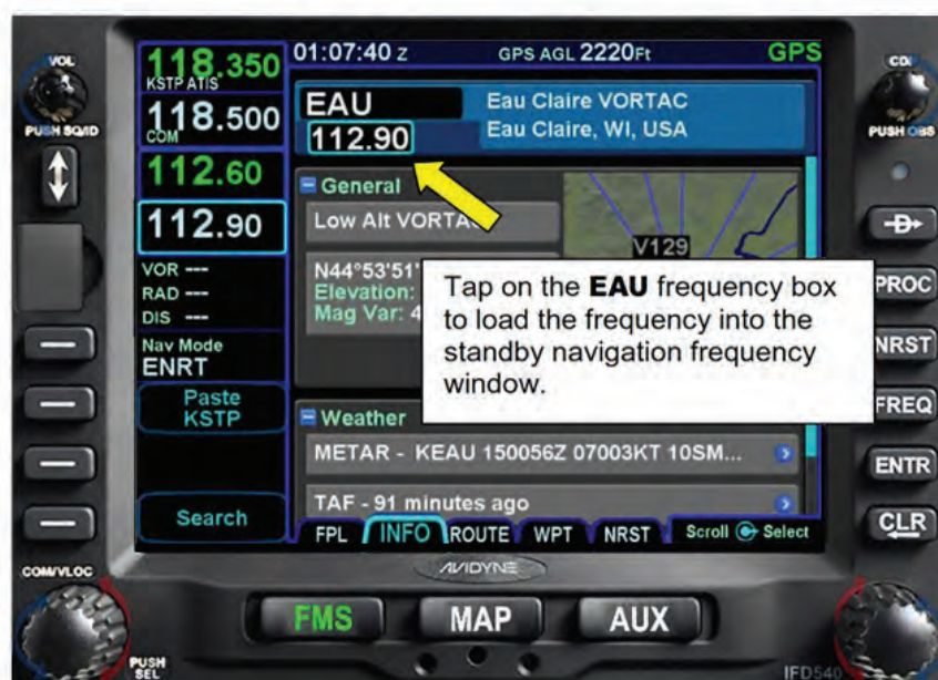
Figure 10 - 14 Loading the EAU VOR Frequency
