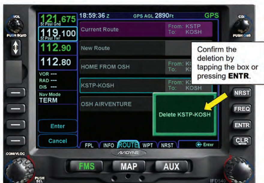
Figure 7 - 21 Confirming the Route Deletion
