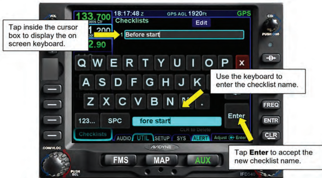
Figure 10 - 33 Entering a New Checklist Name
