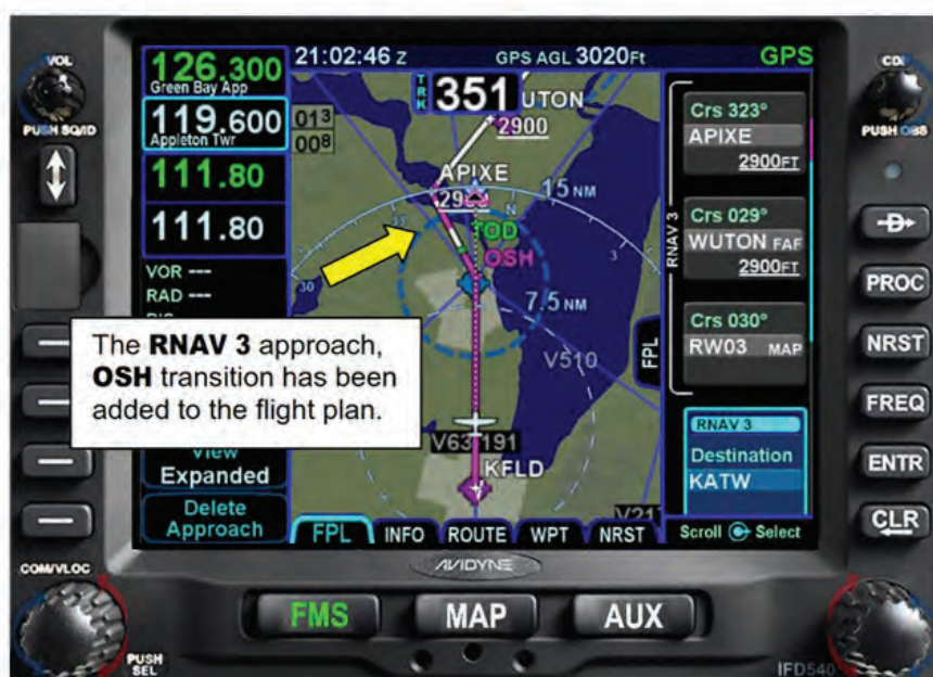
Figure 9 - 10 Flight Plan with RNAV 3 Approach
