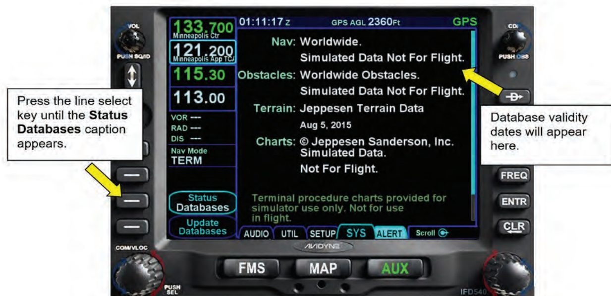
Figure 10 - 42 Displaying Internal Database Information
