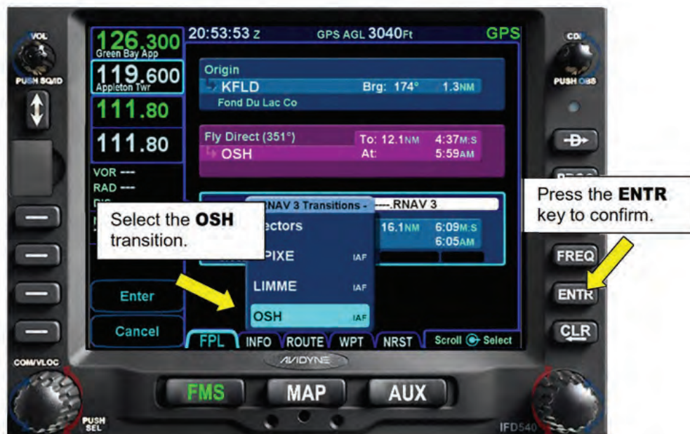
Figure 9 - 9 Selecting the OSH Transition
