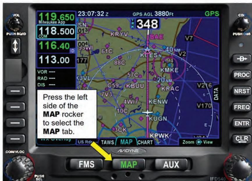
Figure 4 - 15 Using the MAP Rocker
