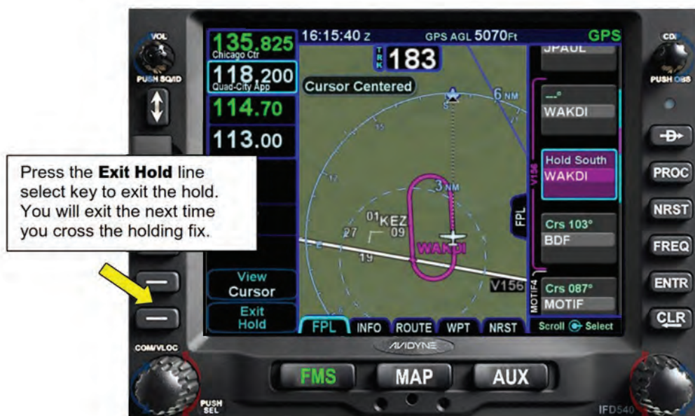
Figure 8 - 13 Exiting the Hold
