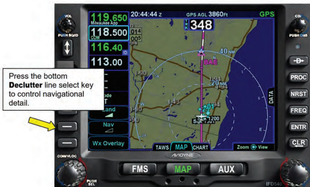
Figure 4 - 23 The Nav De-Cluttering Key
