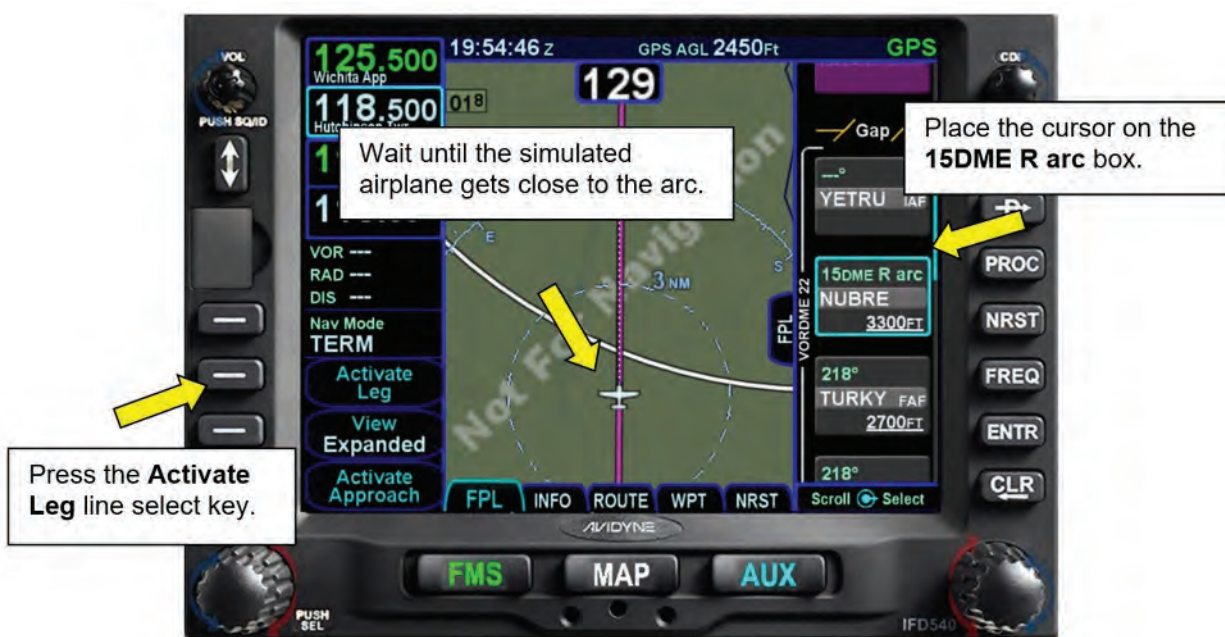
Figure 9 - 36 Intercepting the DME Arc
