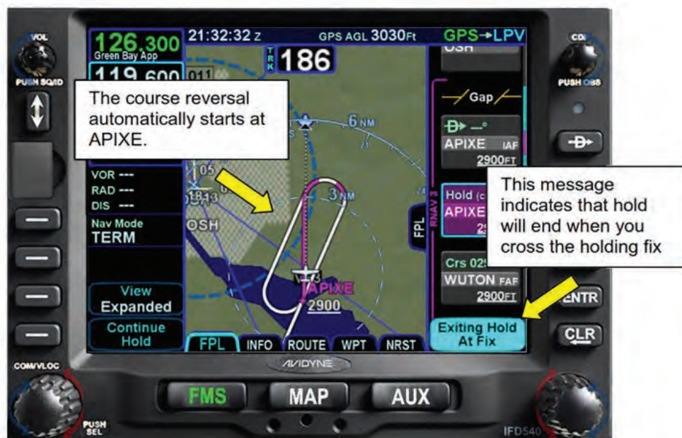
Figure 9 - 18 Entering the Course Reversal Hold
