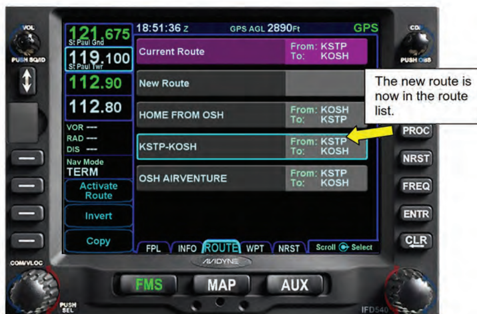
Figure 7 - 16 Route List Showing the New Stored Route
