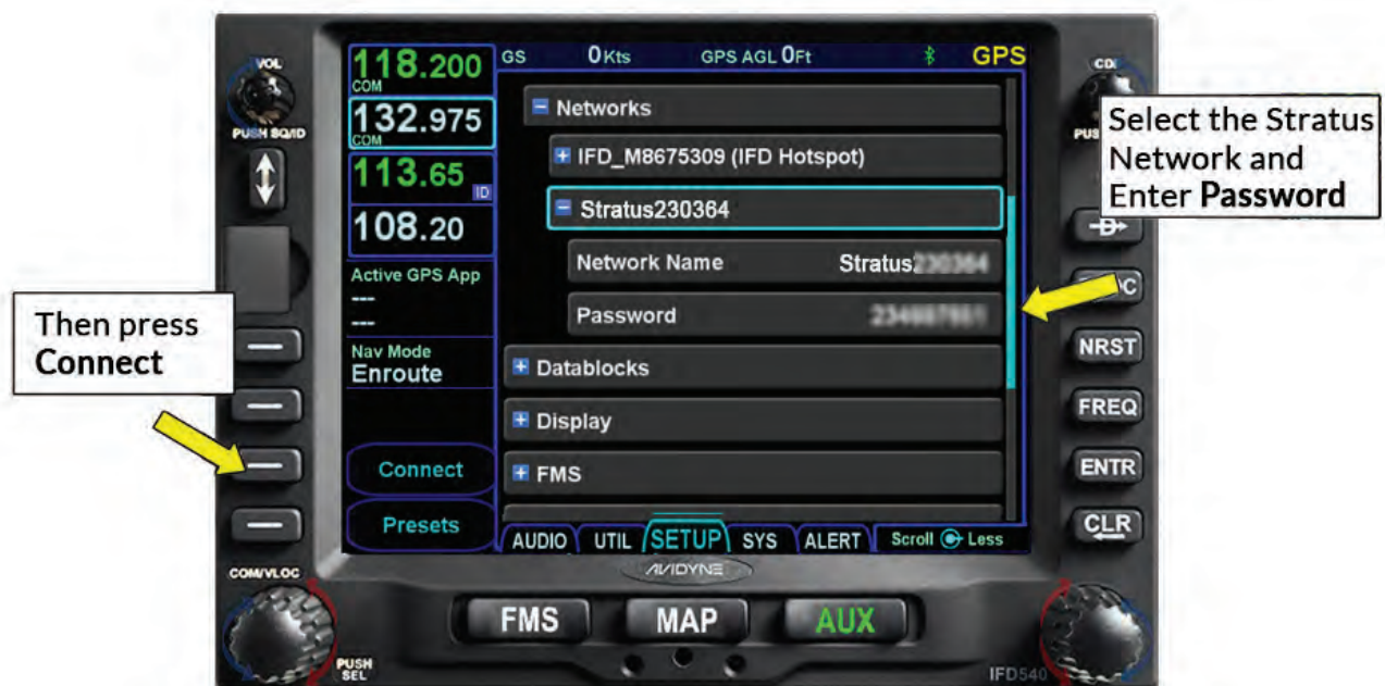
Figure 11 - 41 Connecting the IFD with a portable device such as a Stratus3
