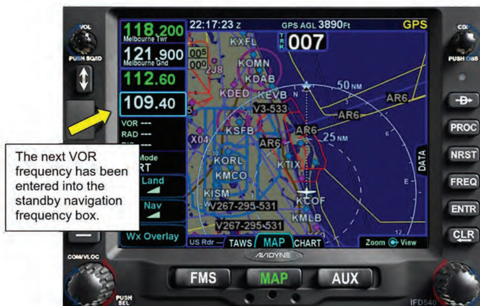
Figure 3 - 11 Setting the Standby Nav Frequency
