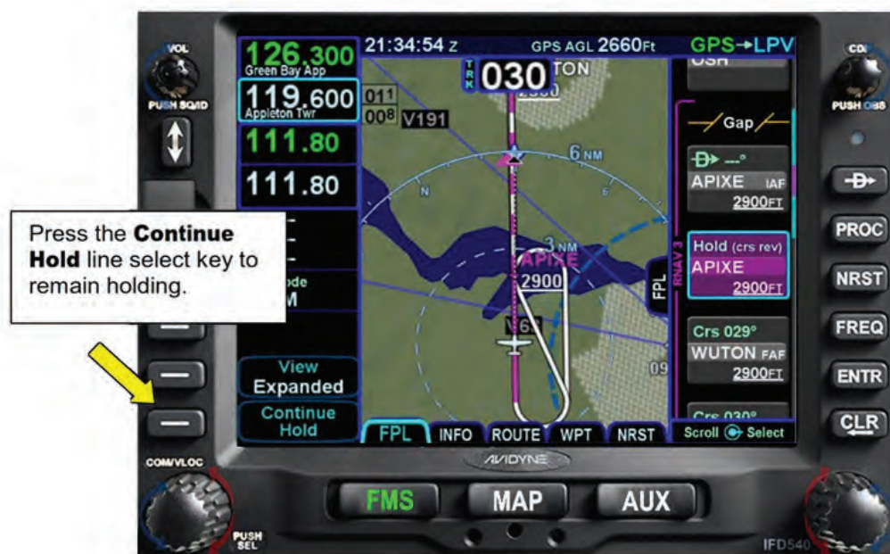
Figure 9 - 19 Proceeding Inbound on the Approach
