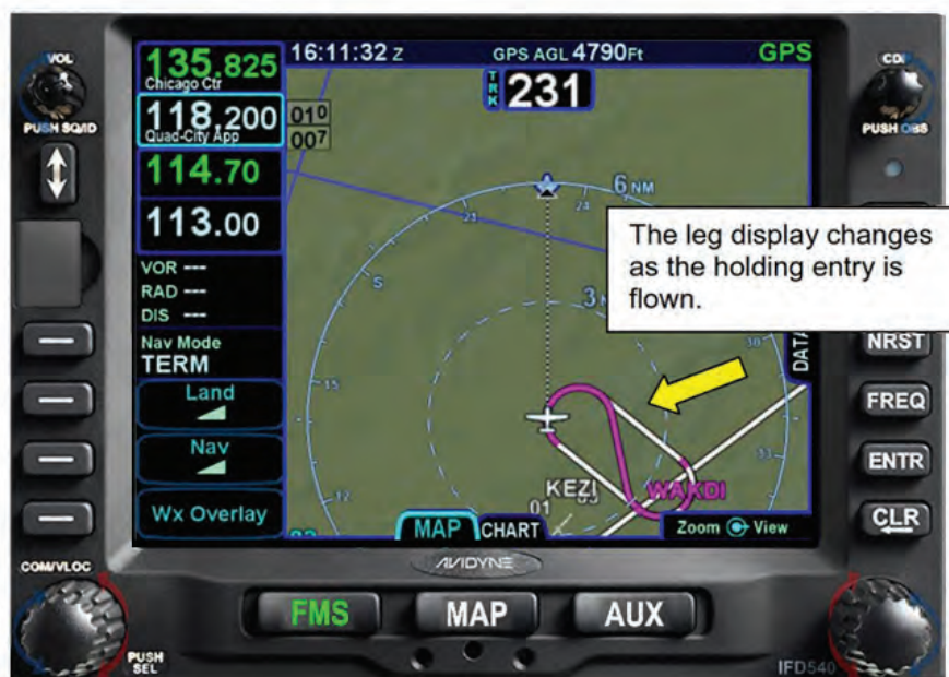
Figure 8 - 11 Entering the Holding Pattern
