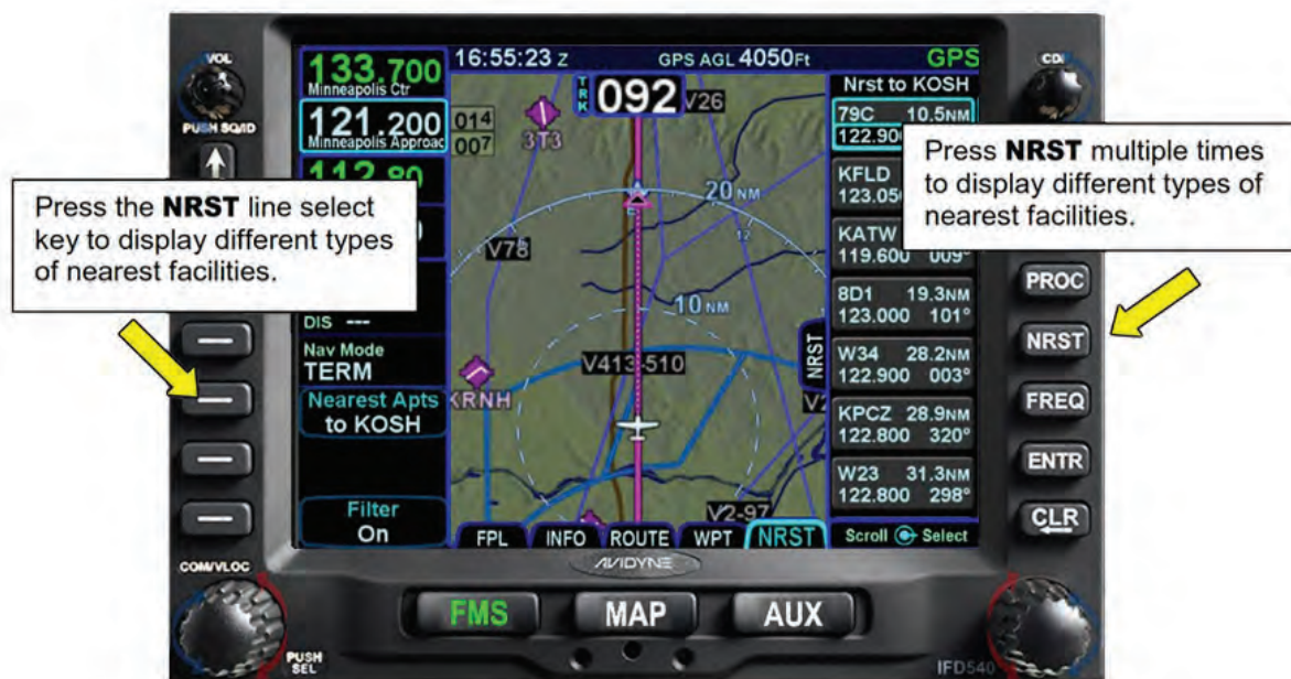
Figure 10 - 23 Displaying Different Types of Nearby Facilities
