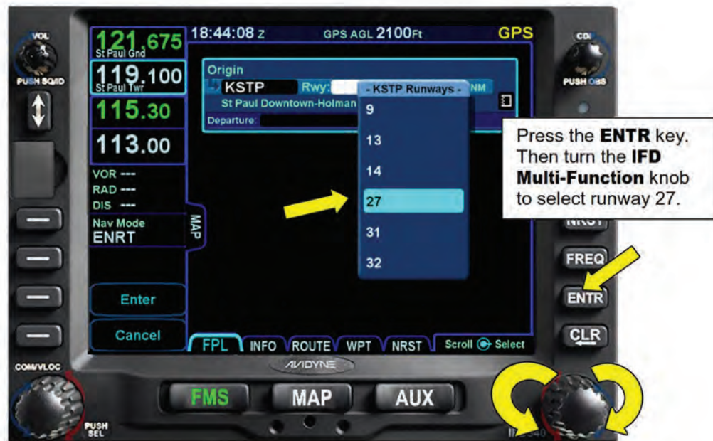
Figure 6 - 13 Selecting the Departure Runway
