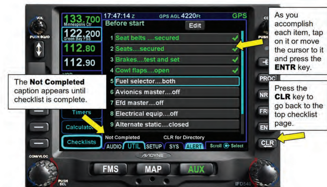
Figure 10 - 39 Using an Electronic Checklist
