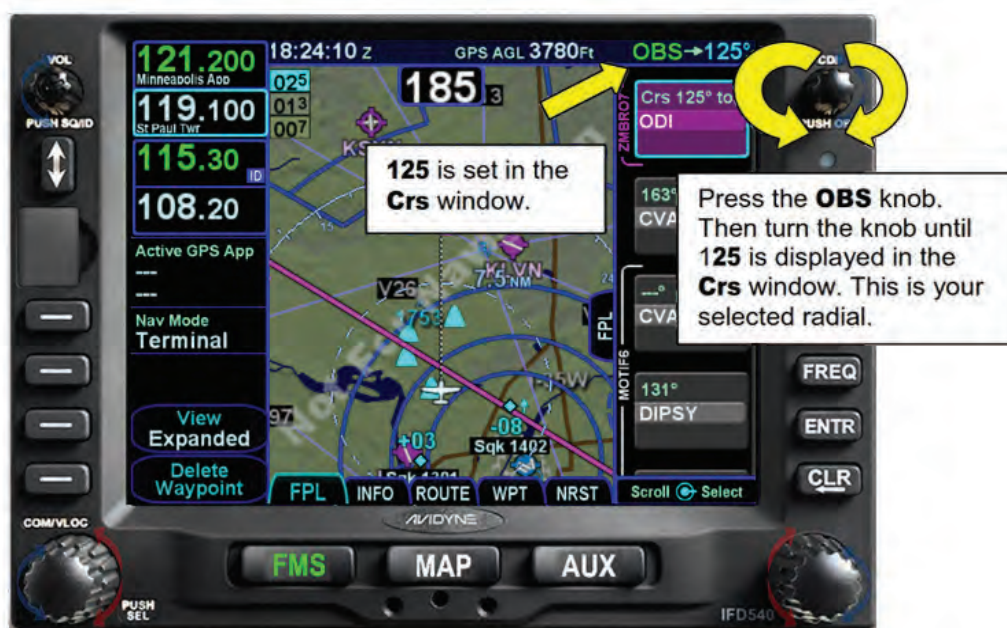
Figure 6 - 33 Setting the Inbound Radial
