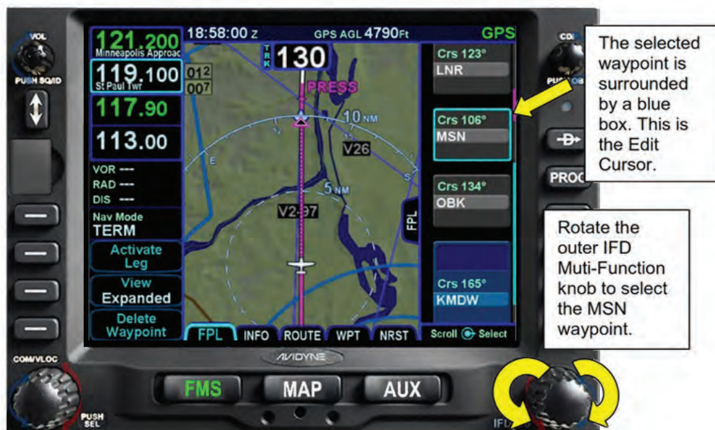
Figure 5 - 6 Selecting the Direct-To Waypoint
