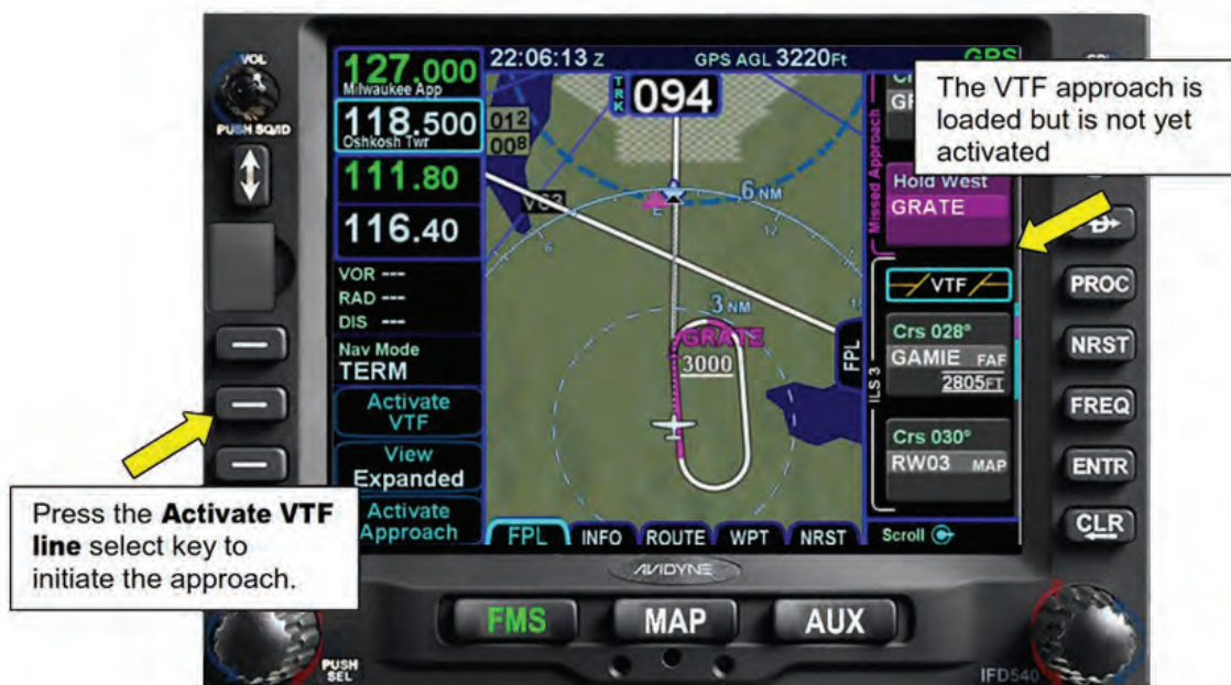
Figure 9 - 28 Activating a Vectors to Final Approach
