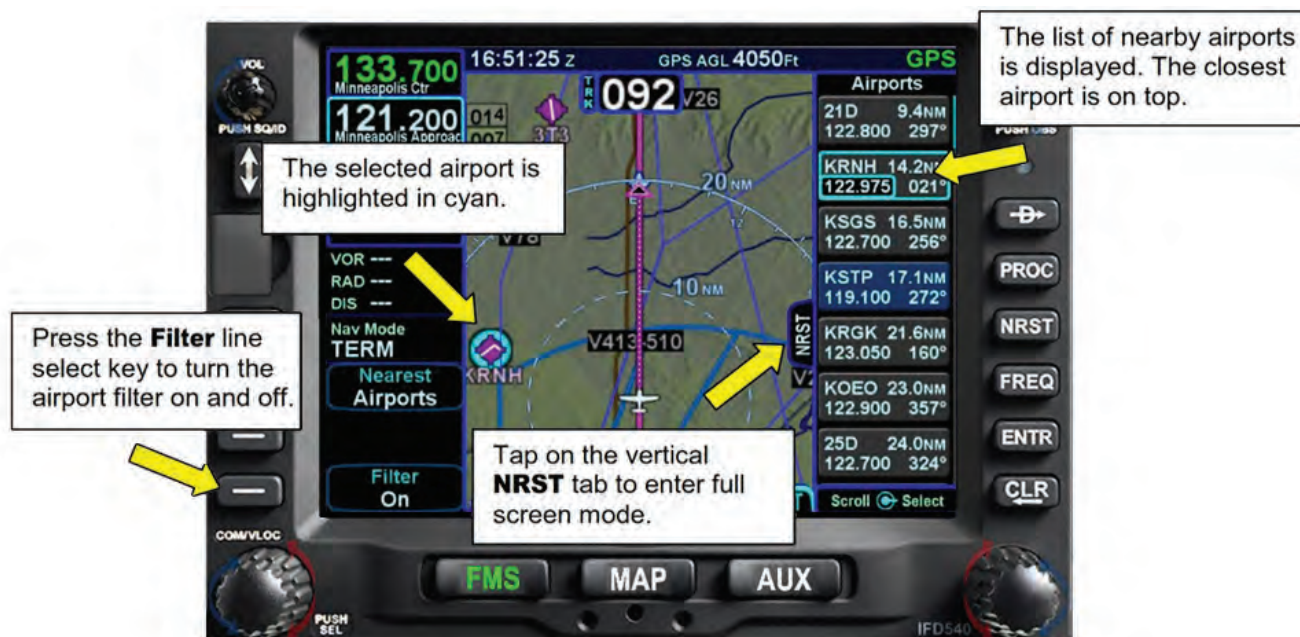
Figure 10 - 20 The NRST Tab
