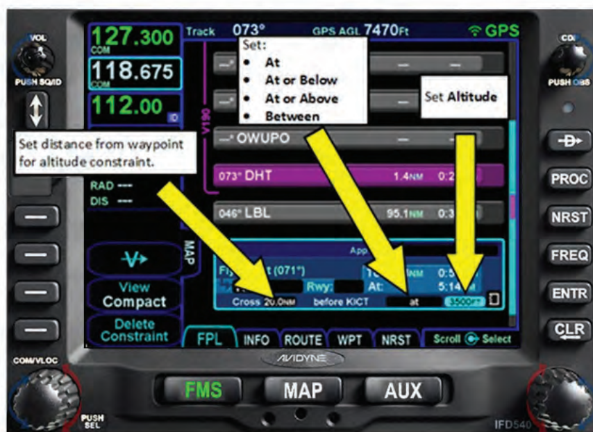
Figure 6 - 44 Setting Altitude Constraint
