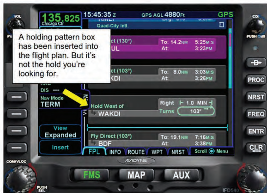
Figure 8 - 4 The New Hold, Before Modification
