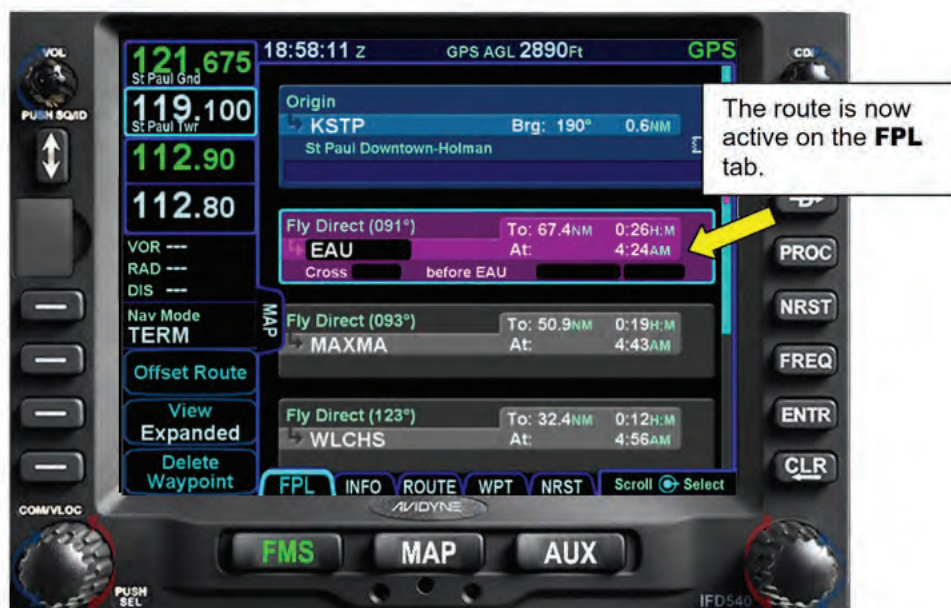
Figure 7 - 19 The Activated Route on the Flight Plan Page
