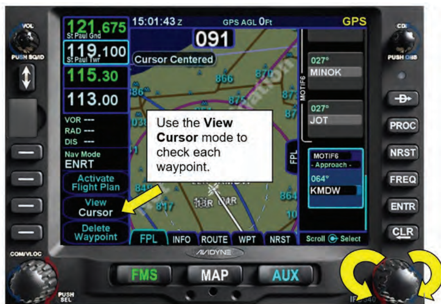
Figure 6 - 25 Using View Cursor to Check the Flight Plan
