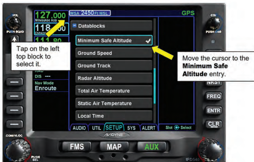
Figure 11 - 9 Setting a New Datablock Value
