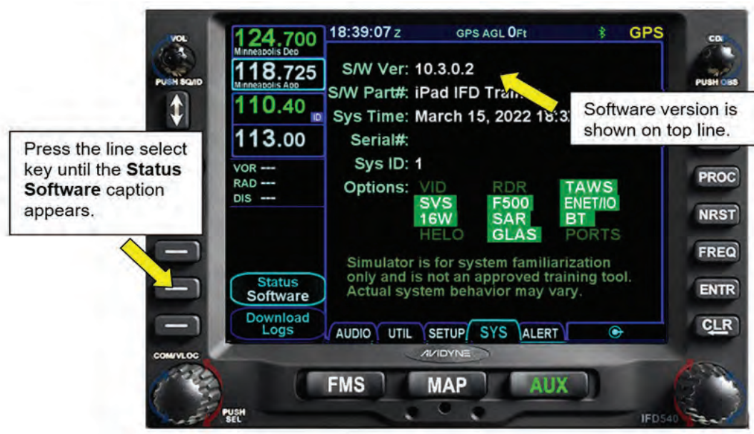
Figure 10 - 41 Displaying Software Version Information
