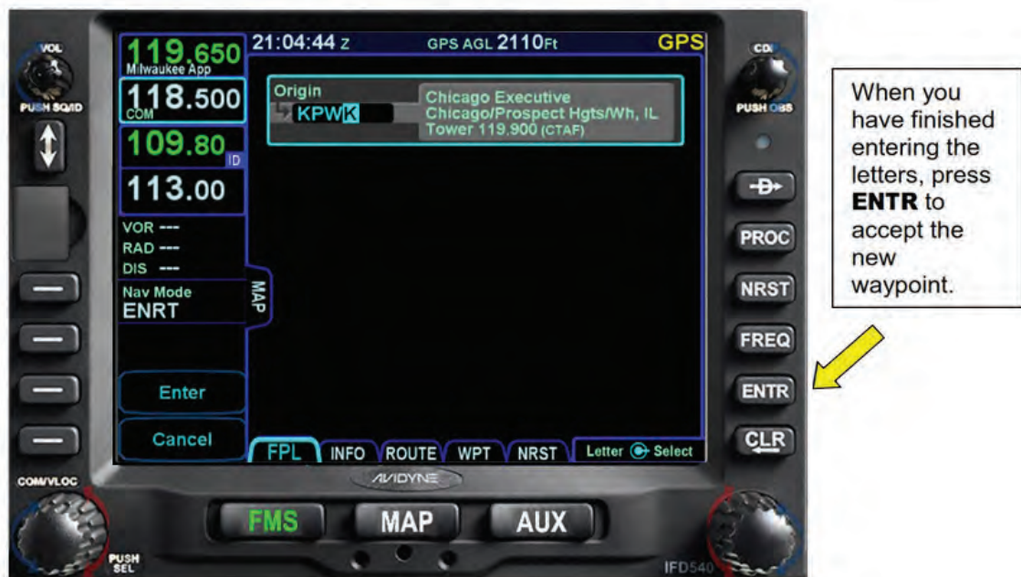
Figure 4 - 6 Press ENTR to Accept the Origin
