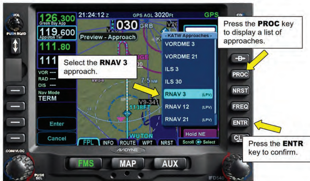
Figure 9 - 14 Selecting the RNAV 3 Approach
