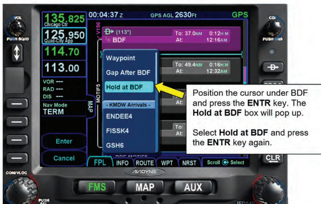
Figure 8 - 17 Programming the Hold at BDF
