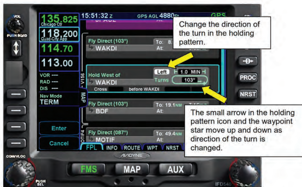
Figure 8 - 6 Modifying the Holding Pattern
