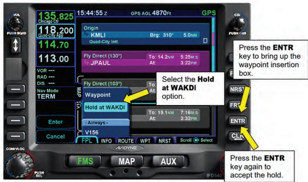
Figure 8 - 3 Inserting the Hold into the Flight Plan
