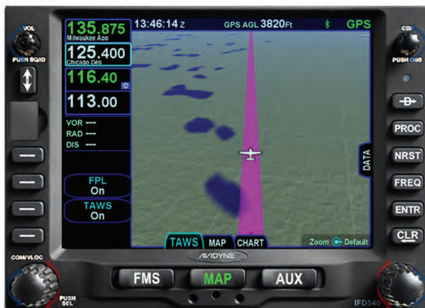
Figure 4 - 30 TAWS tab - Datablocks off
