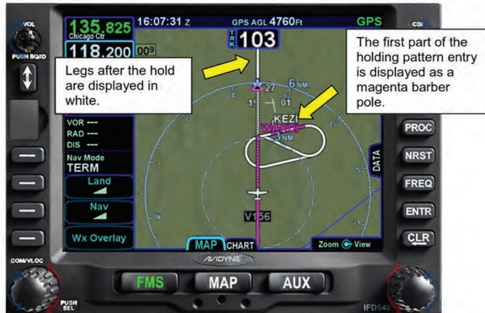
Figure 8 - 9 Holding Pattern Components
