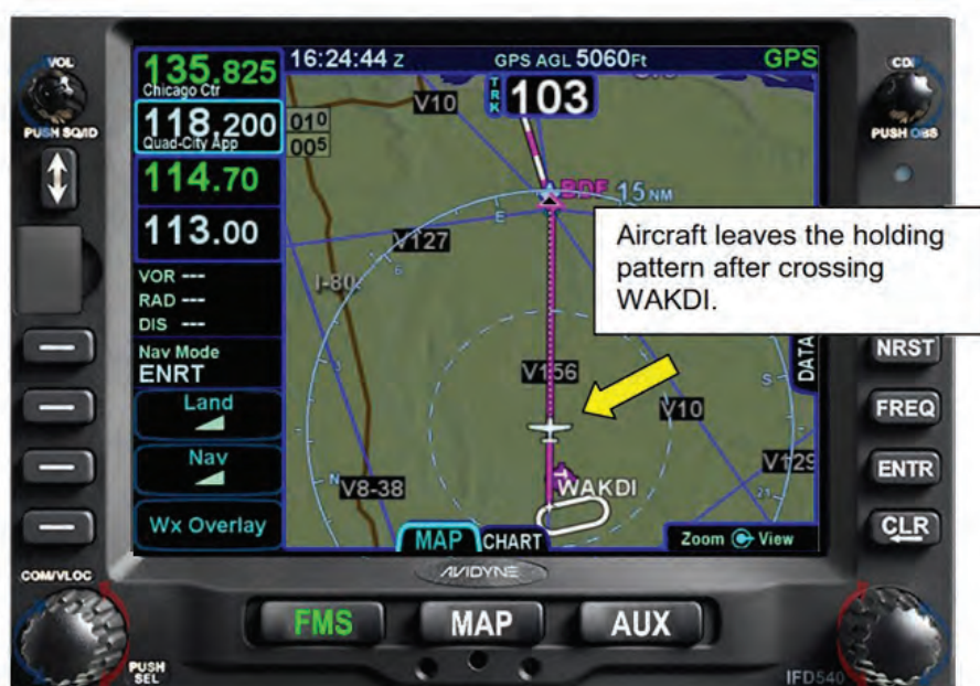
Figure 8 - 15 After the Holding Pattern Has Been Exited
