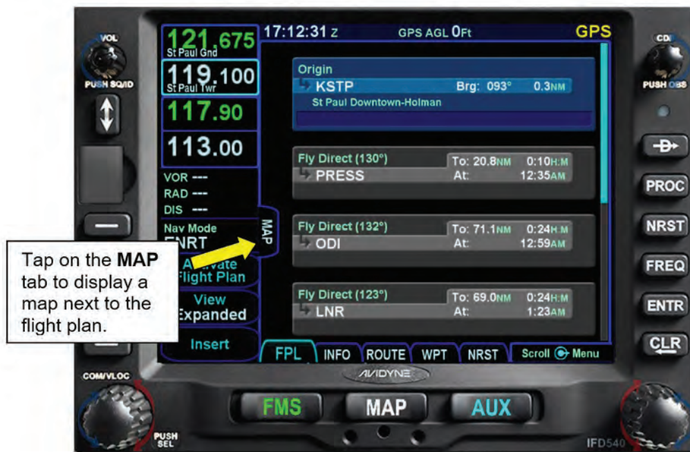
Figure 5 - 3 Opening the Flight Plan MAP Tab
