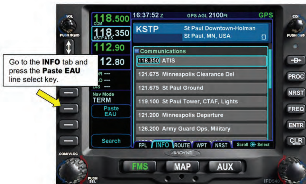
Figure 10 - 13 Pasting EAU into the INFO Tab
