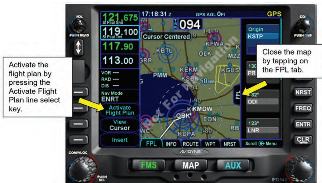
Figure 5 - 5 Closing the Flight Plan MAP Tab
