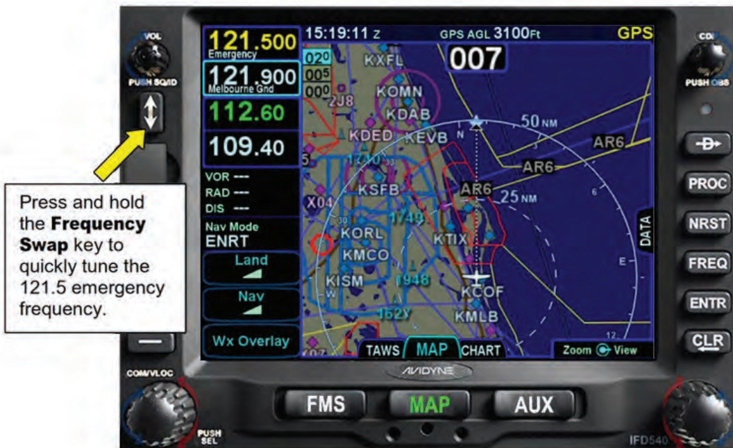
Figure 3 - 15 Quick-Tuning the 121.5 Emergency Frequency
