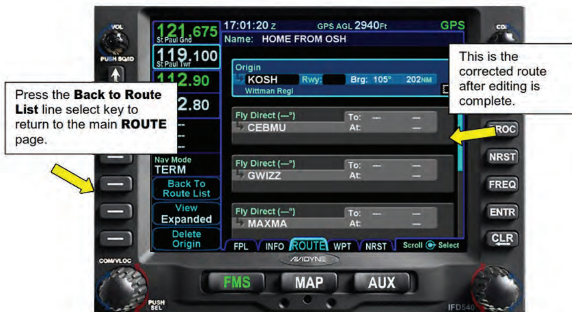
Figure 7 - 12 The Corrected Route
