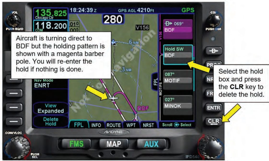
Figure 8 - 23 Exit Step 2: Delete the Hold
