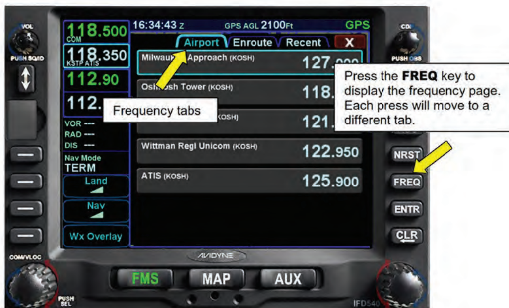
Figure 10 - 11 Using the FREQ Key
