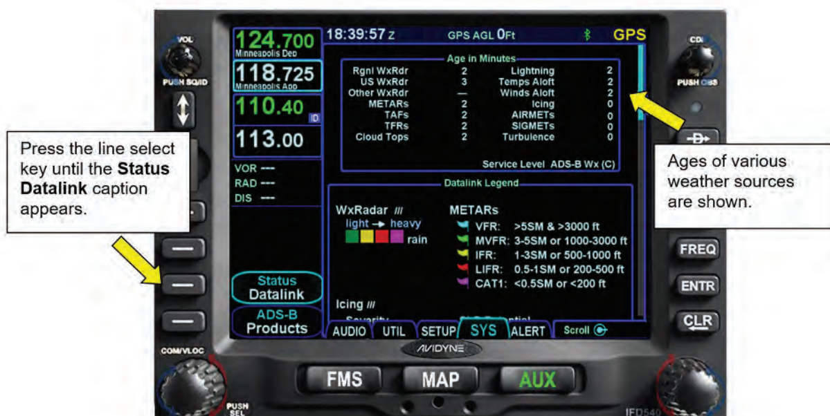
Figure 10 - 44 Displaying Datalink Information
