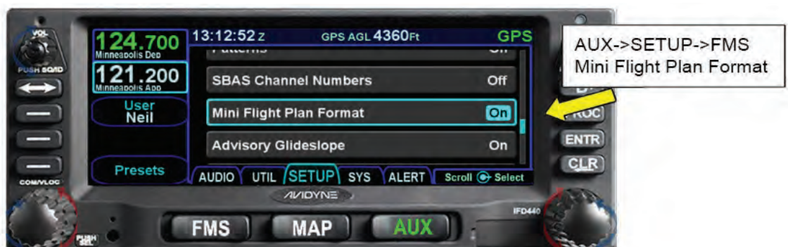
Figure 11 - 45 Selecting Mini Flight Plan Format
