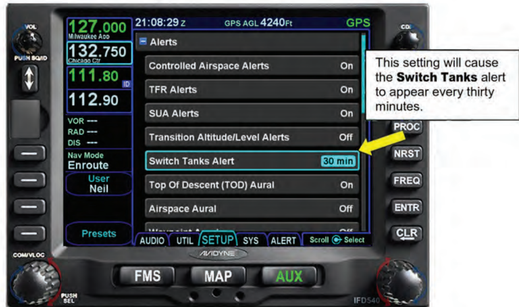
Figure 11 - 27 Setting the Switch Tanks Alert
