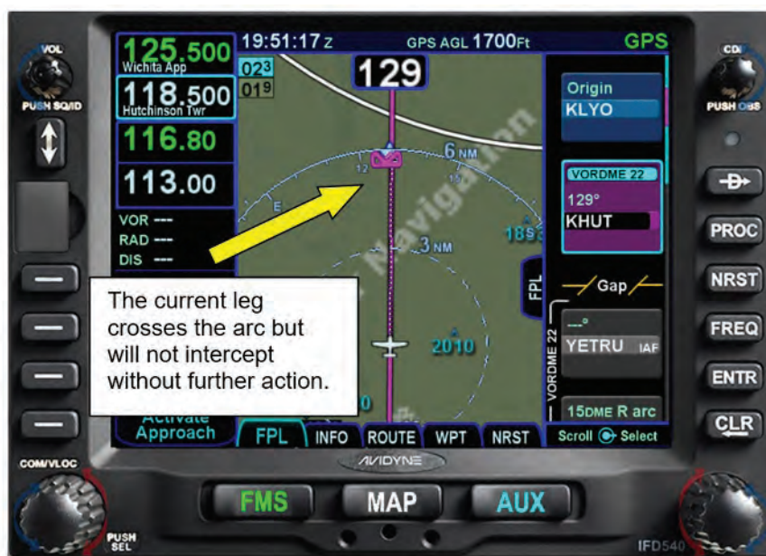
Figure 9 - 35 The Current Flight Plan and the DME Arc
