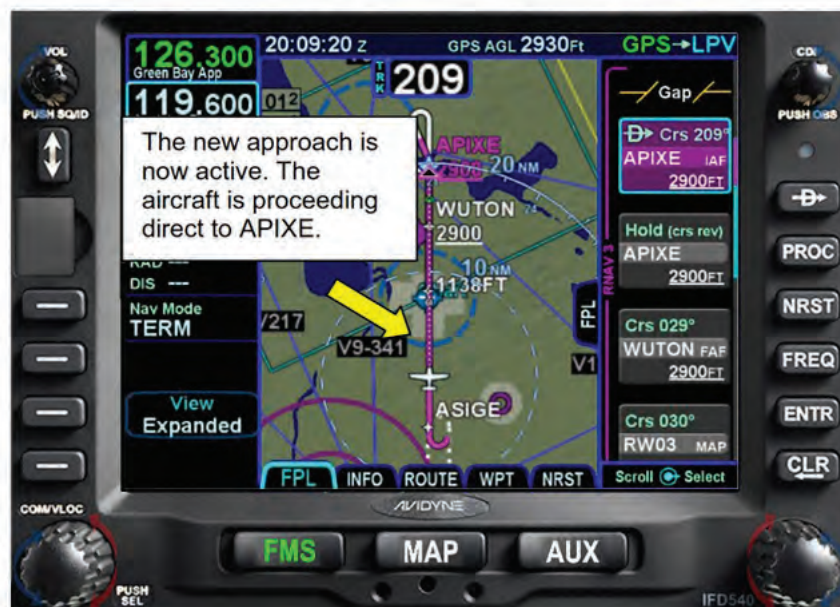
Figure 9 - 17 Starting the New Approach
