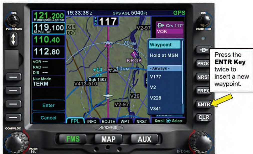
Figure 5 - 18 Inserting a New Waypoint
