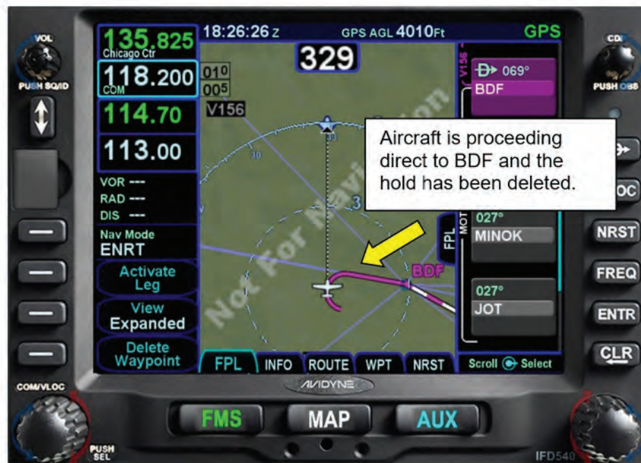
Figure 8 - 24 Updated Flight Plan After Hold is Deleted
