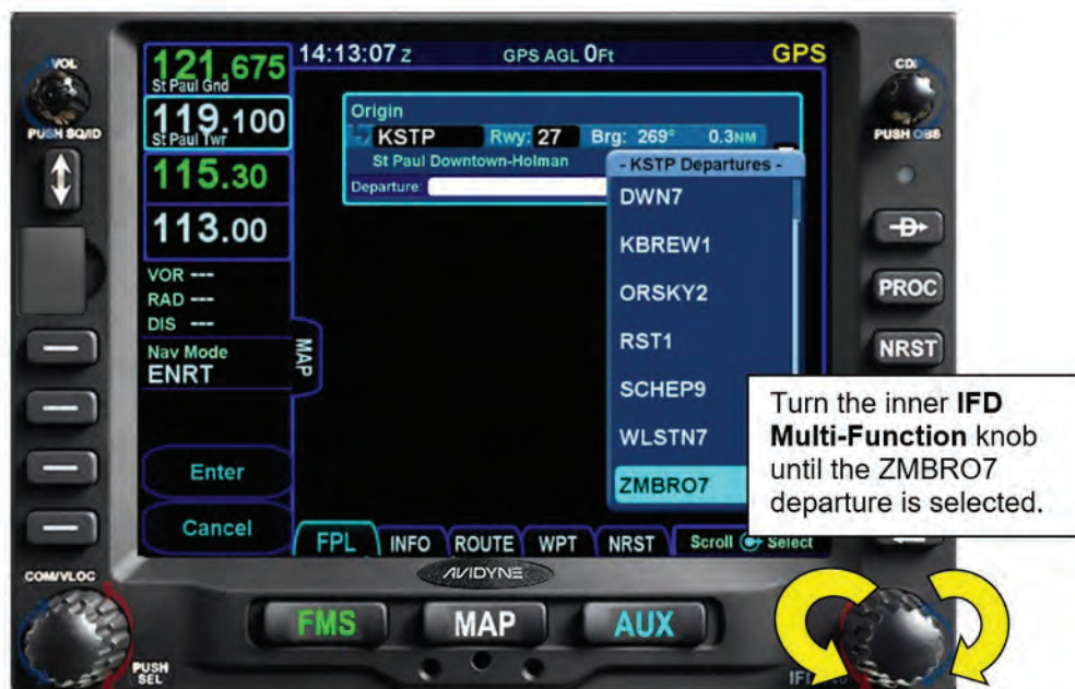
Figure 6 - 17 Selecting the Departure Procedure
