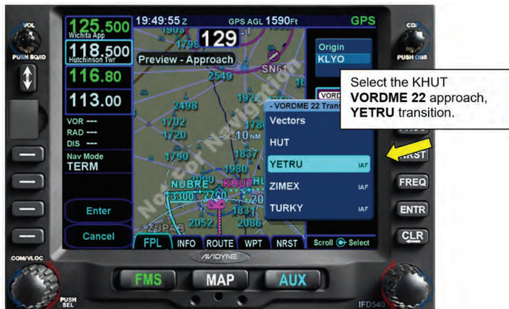
Figure 9 - 34 Selecting the VOR/DME 22 Approach to KHUT
