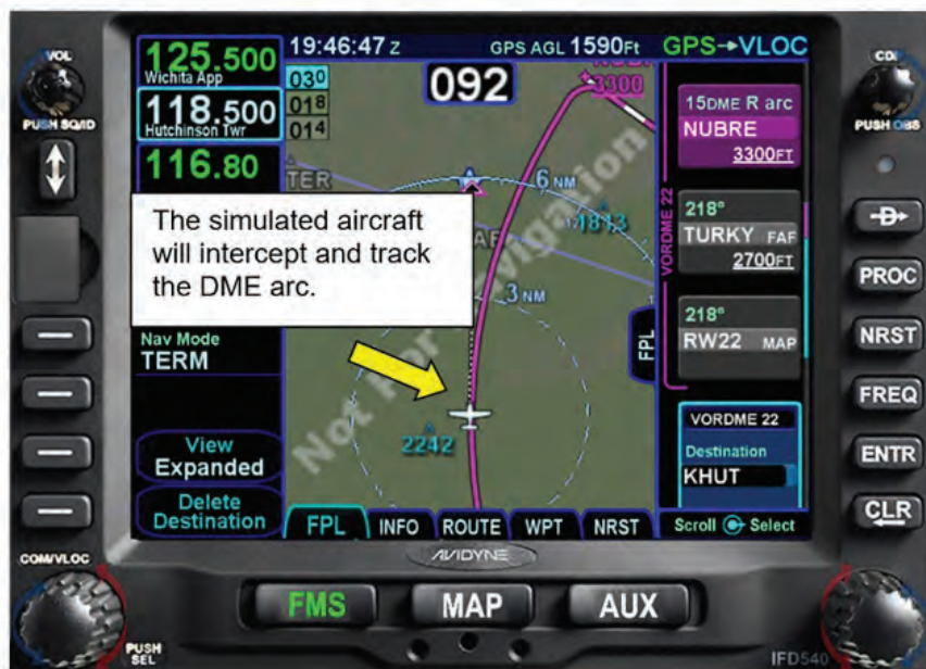
Figure 10 - 1 Selecting the FMS INFO Tab
