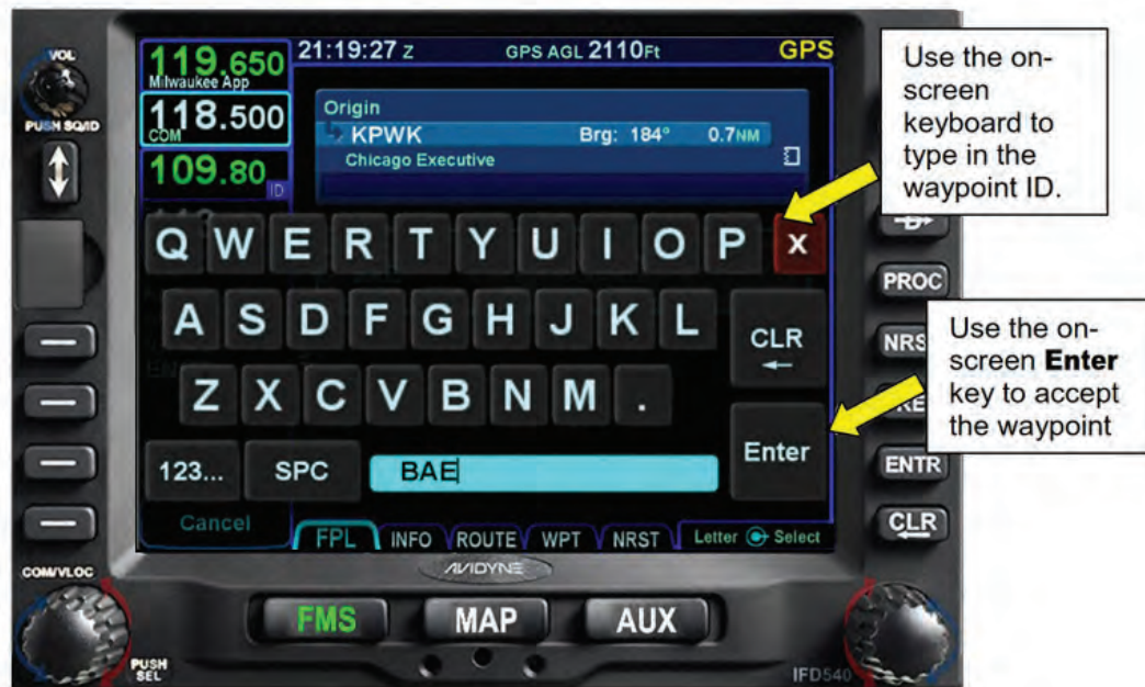
*Figure 4 - 11 Using the On Screen Keyboard to Enter a Waypoint
