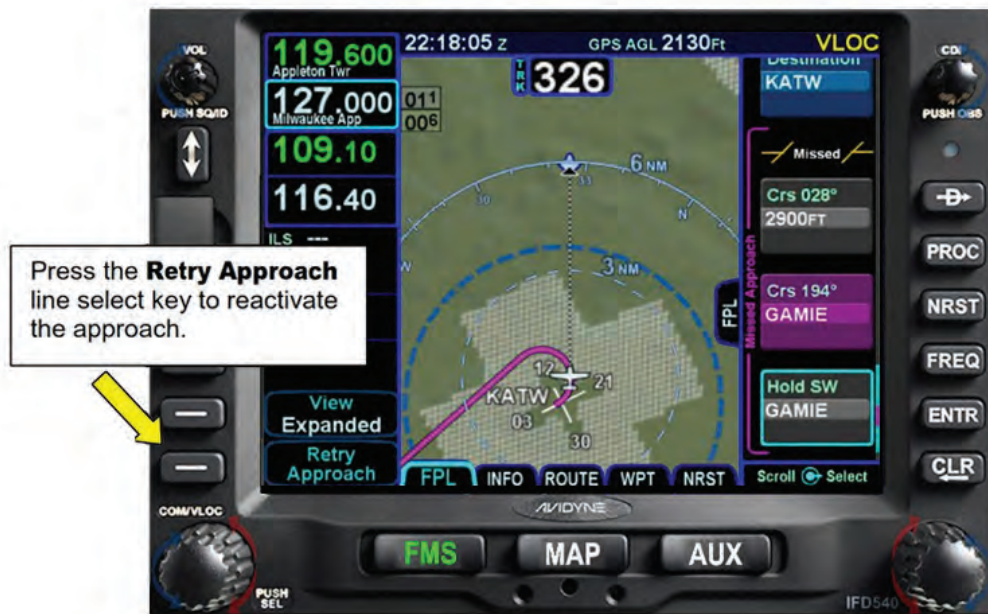
Figure 9 - 31 The Retry Approach Line Select Key
