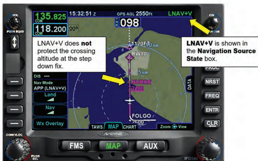
Figure 9 - 4 IFD540 Showing LNAV+V Approach
