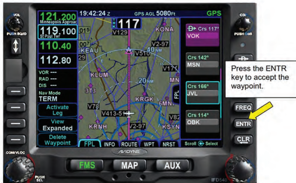
Figure 5 - 20 Accepting the Inserted Waypoint
