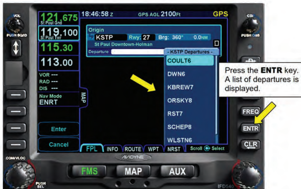
Figure 6 - 16 Displaying the List of Departures
