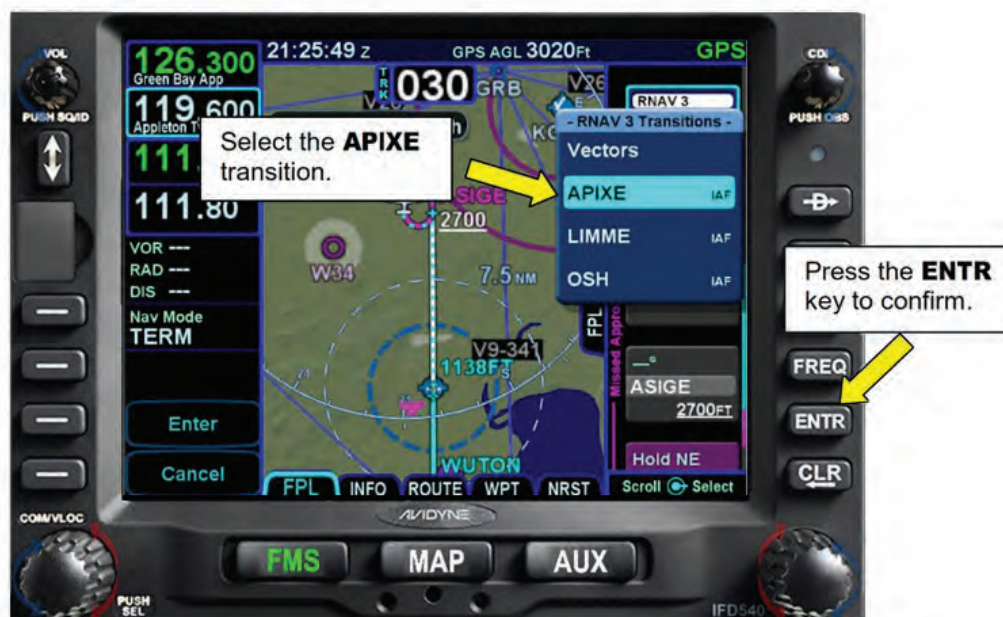
Figure 9 - 15 Selecting the APIXE Transition
