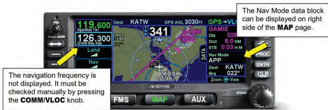
Figure 9 - 42 IFD440 Approach Indications
