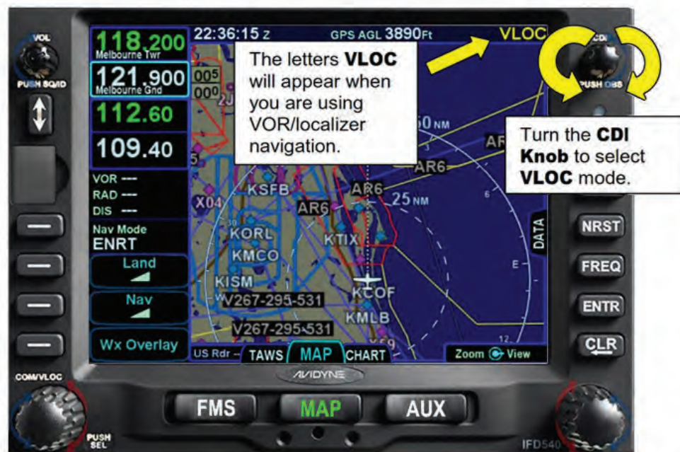
Figure 3 - 12 Changing to VLOC Navigation
