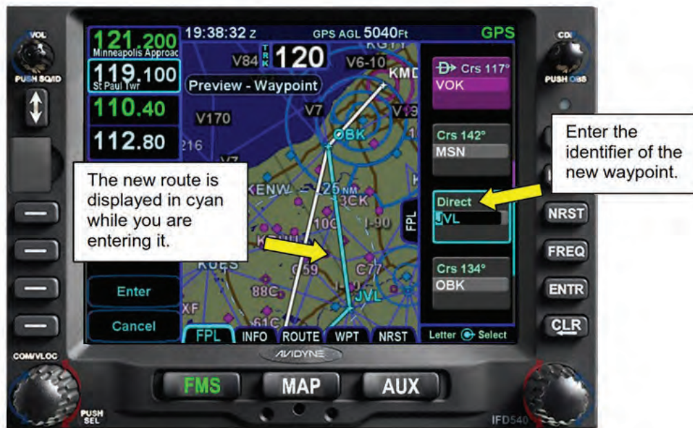
Figure 5 - 19 Entering the Waypoint Identifier
