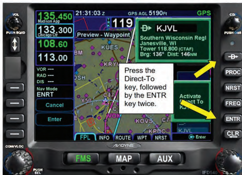
Figure 5 - 25 Activating the Direct-To Destination
